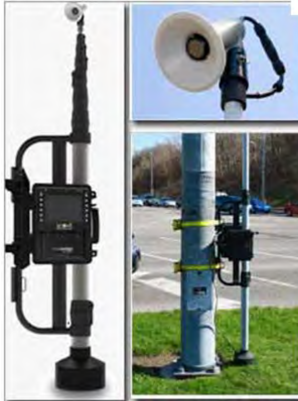
Exhibit 3-1. Automated intersection count station.
