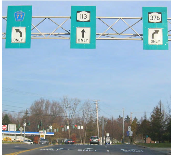
Exhibit 5-22. Example of advance overhead signs and pavement markings indicating lane use for various destinations.
