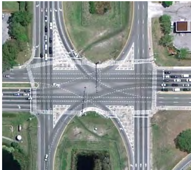
Exhibit 4-6. Single point urban intersection (SPUI) with pavement marking delineation for turning movements.
