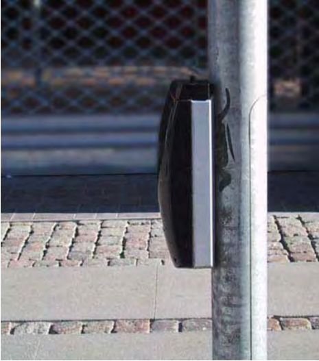
Figure 10-15. The tactile arrow on the APS in Denmark was on top of the device, which was located on a pole near the crosswalk line. Most intersections were pretimed, so no pushbutton was included on this device.
