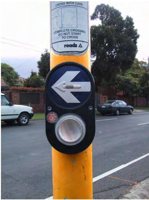
Figure 10-7. This APS has a tactile arrow within a larger visible arrow. A raised bar on the tactile arrow indicates that this is an APS. Other features include a locator tone and audible and vibrotactile “Walk” indication.
