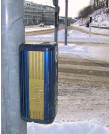
Figure 10-12. The Swedish APS displays a tactile map on one side.
