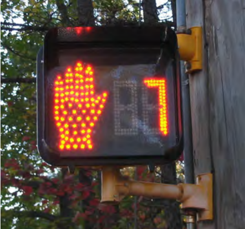
Figure 3-8. Correct display of pedestrian countdown signal (counting down during flashing “Don’t Walk”).
