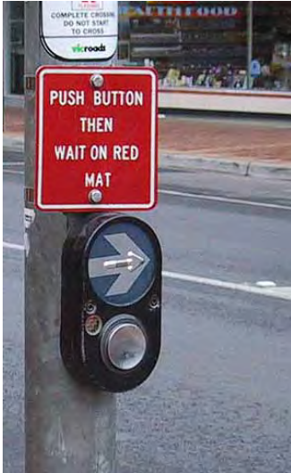
Figure 4-10. Detail of an APS at midblock crossing in Australia. Sign reads “Push button then wait on red mat.”
