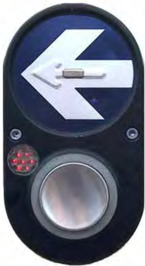
Figure 4-5. A red actuation light is near located just above and to the left of the pushbutton.
