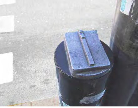
Figure 10-16. Danish APS with tactile bar (arrow) mounted on the top. The bar is aligned with the crosswalk, and two knobs at the end of the bar indicate a median and the far side of the street.
