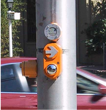
Figure 6-22. The direction of the cast-in-place arrow on this device must be specified when ordering.
