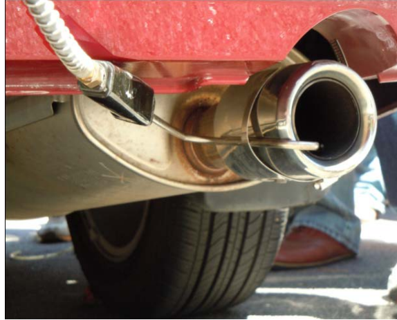
Figure 2. Photo. Illustration of PEMS tailpipe emissions measurement (for additional details on PEMS see [2]).
