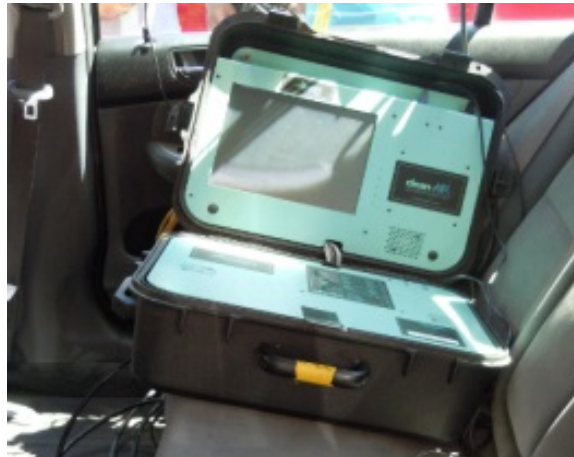
Figure 3. Photo. Illustration of PEMS computer recording unit (for additional details on PEMS see [2]).
