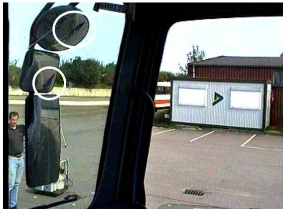
Fig 28: Picture showing the driver's view from the Mercedes Benz MIM vehicle of the cyclist in the corner impact scenario, s = 18.5 m before impact, Test 8
