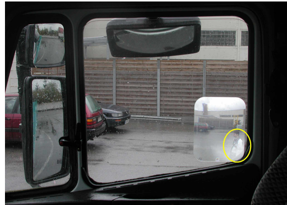
Fig 20: Picture showing the resulting view cone from the front mirror (MB MIM vehicle)
