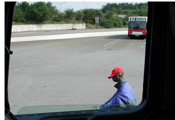
Fig 30: Picture showing the driver's view from the Mercedes Benz MIM vehicle when the cyclist appears in the direct field of view of the driver of the Mercedes Benz 1748 for the first time, s = 5.9 m before impact, Test 8
