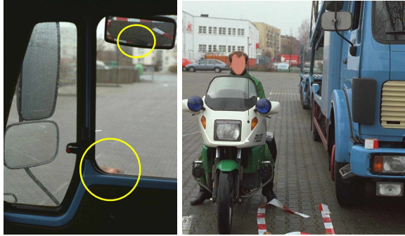
Fig 13: An example of the right-handed arrangement of mirrors on a truck (top of hair visible)
