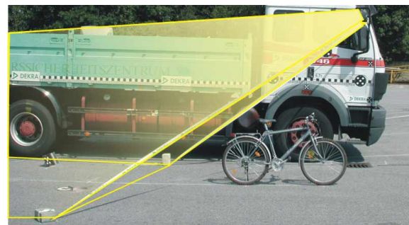
Fig 17: Photo showing the indirect field of view from the driver's viewpoint (MB 1748) via the wide-angle mirror (the overlay pyramid stump marks the coverage of the wide-angle mirror; the cycle is located 2.0m away to the truck.)
