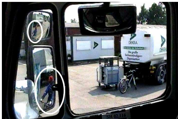
Fig 27: Picture showing the driver's view from the Mercedes Benz 1748 of the cyclist for the side impact scenario, impact scenario Test 7
