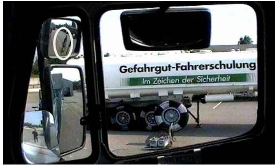
Fig 26: Picture showing the driver's view from the Mercedes Benz 1748 of the cyclist in the side impact scenario, s = 16.5 m before impact, Test 7
