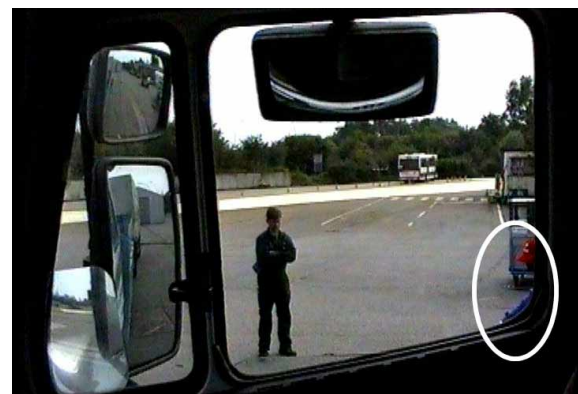
Fig 25: Picture showing the driver's view from the Mercedes Benz 1748 when the cyclist appears for the first time in the field of vision of the driver of the Mercedes Benz 1748, s = 5.9 m before impact, Test 6
