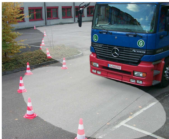
Fig 32: Field of view via the wing mirror in the DaimlerChrysler MIM vehicle /2/
