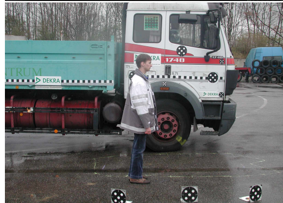
Fig 21: Picture of the indirect field of view (Mercedes Benz 1748) on the front right-hand side upon the fitting of a standard Fresnel lens in the rear part of the right-hand side window, person only visible with Fresnel lens, marking plates define the beginning of the field of view of the Fresnel lens on the ground.
