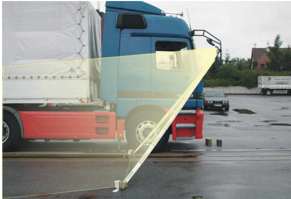
Fig 18: Picture showing the indirect field of view from the driver's viewpoint (Mercedes Benz MIM vehicle) via the wide-angle mirror; the marking tape defines the lower limit of coverage in the mirror and the key points of the actual field of view on the ground.
