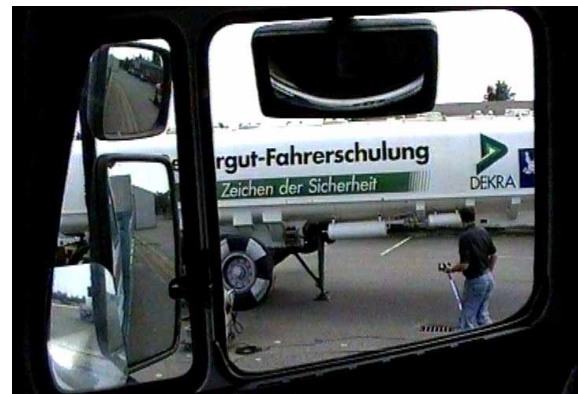
Fig 24: Picture showing the driver's view from the Mercedes Benz 1748 of the (not visible) cyclist for the corner impact scenario, s = 17.1 m before impact, distance of cyclist-truck a = 3.5 m, Test 6
