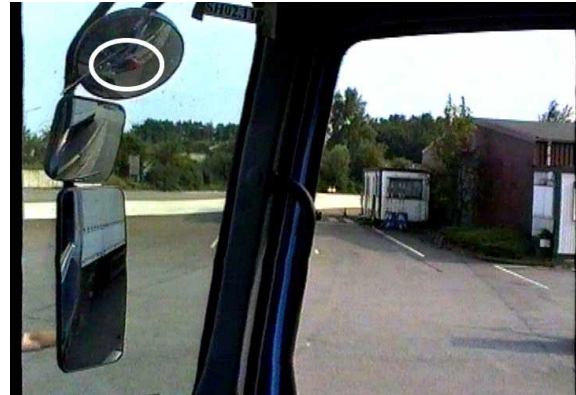
Fig 29: Picture showing the driver's view from the Mercedes Benz MIM vehicle of the cyclist in the corner impact scenario, impact scenario, Test 8
