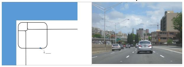
Description: This portion of the Factiuousville Beltway has 4 lanes in each direction and closely spaced cloverleaf interchanges with local arterials. The high density of interchanges can negatively impact operations with vehicles weaving to enter and exit the freeway. The probe data reflects a segment between a set of the cloverleafs.
