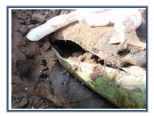
Figure 1 – Failed Pipe Joint
