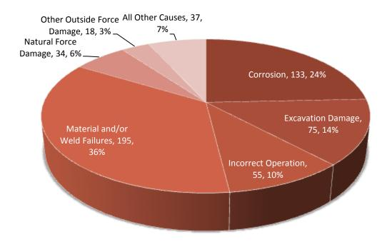
Figure 1 Causes of Significant Onshore Hazardous Liquid Pipeline Incidents
