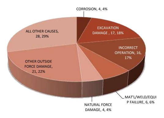
Figure 3 Significant Distribution System Incidents by Cause (2008-2010)
