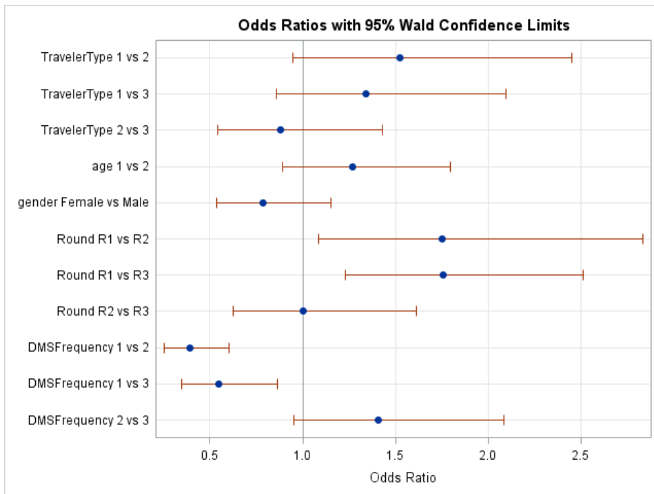
Figure C-16. Graph. Odds Ratios with 95 Percent Confidence Limits – Behavior Hypothesis on whether Safety-Related DMS Cause Drivers to Slow Down in Missouri.
