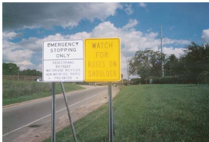
Figure 42. Photo. MnDOT on-ramp Bus-on-shoulder warning sign, right side of photo. (Source: TCRP Report 151)
