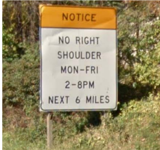
Figure 62. Photo. Notice informing motorists of the lack of right shoulder during shoulder running operations, I-66 mainline.
