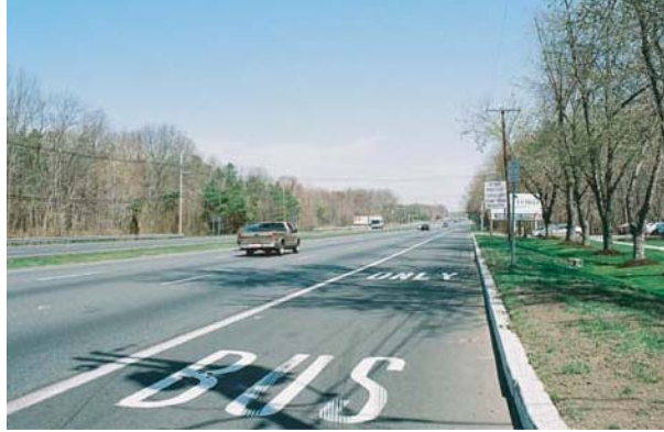
Figure 45. Photo. NJDOT word pavement markings for BOS operation.
