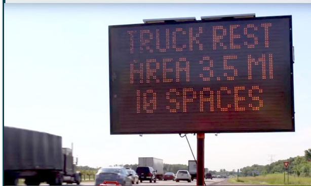
Figure 10. Photo. Variable message sign information display from Minnesota SmartPark system.
