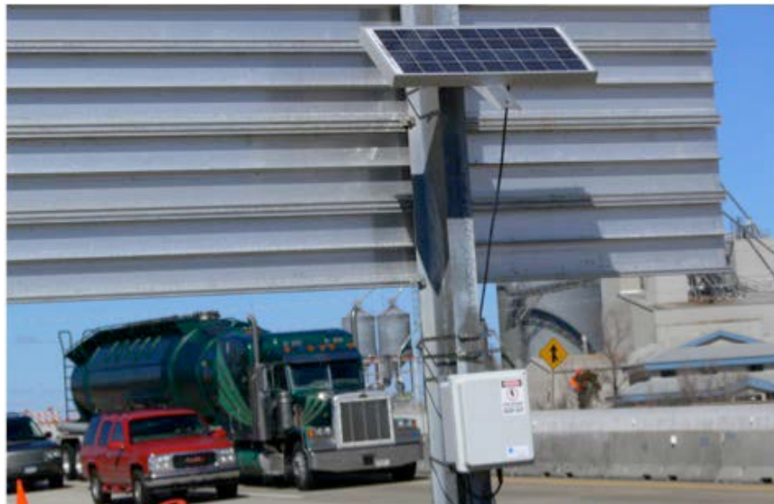
Figure 1. An Example of a Roadside Bluetooth Detector
