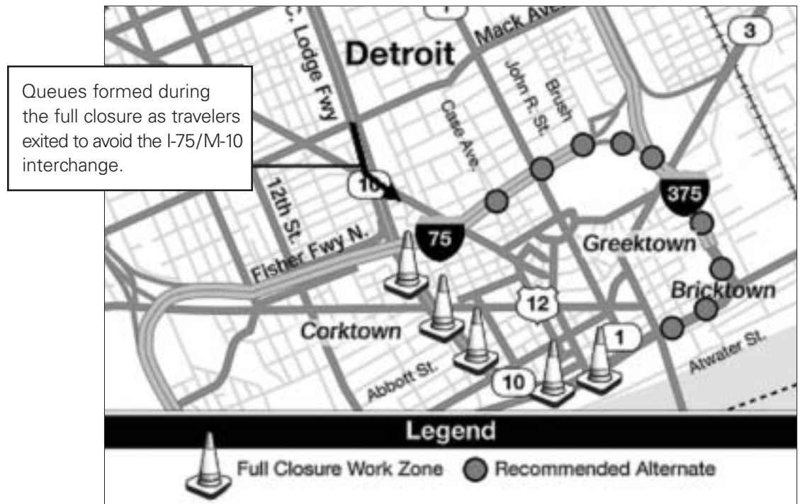
Figure 3 – Delays occurred off of one exit during the full closure
