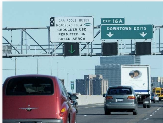
Figure 5. Minnesota: priced dynamic shoulder lane on I-35.
