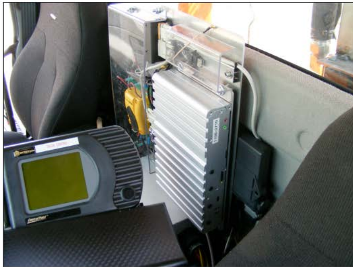
Figure 2: A complete AT500 installation, as seen from the operator's side.
