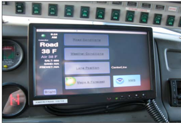
Figure 10: The AT500's MDT displaying the Main Screen.
