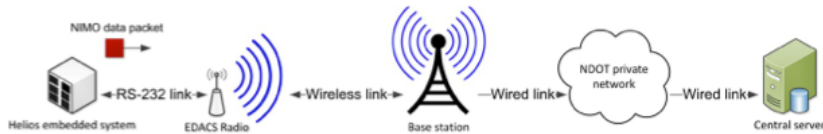
Figure 11. Helios embedded system-to-central server communication links.
