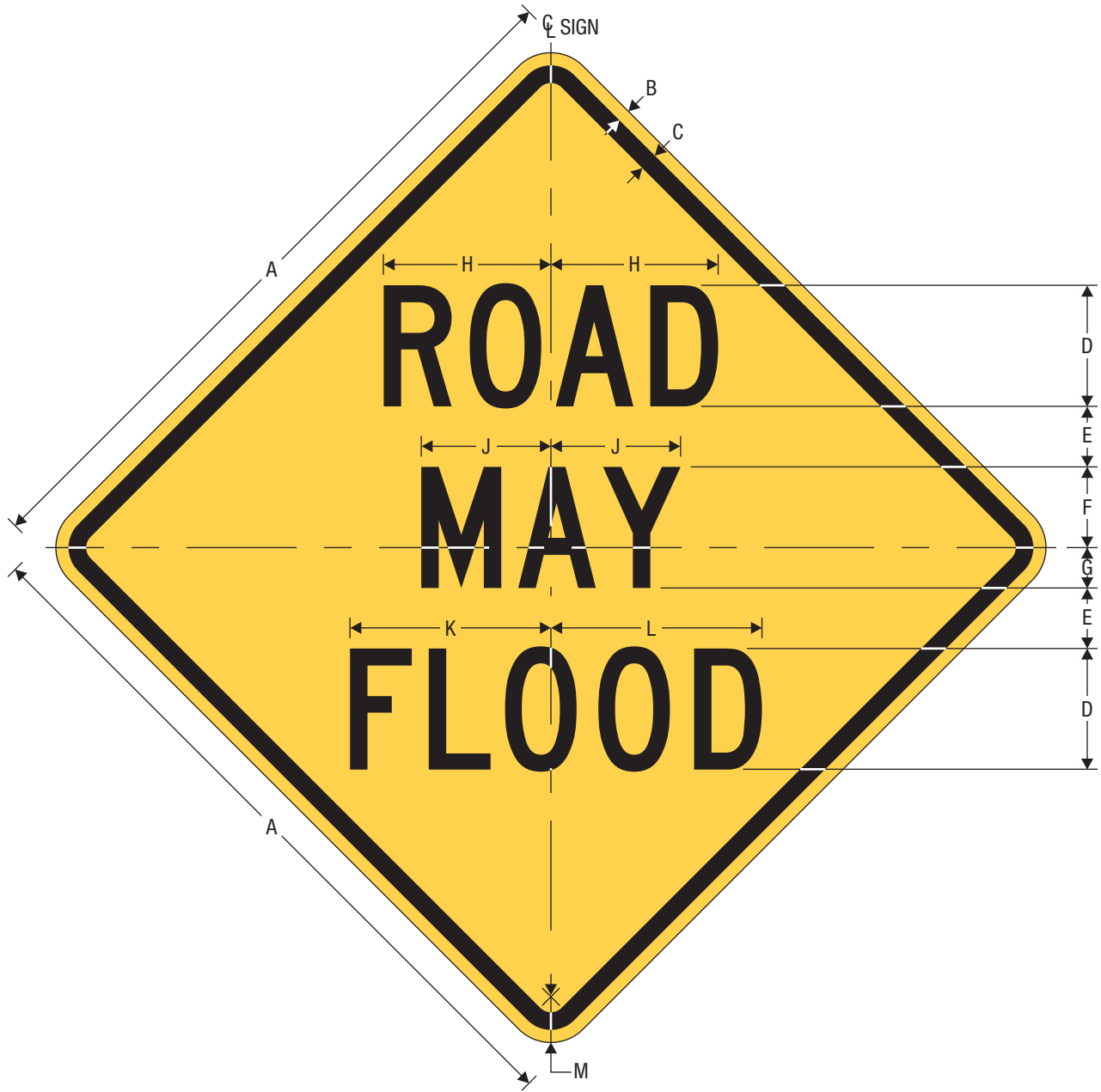
W8-18 ROAD MAY FLOOD
