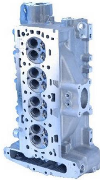
Figure 5.19 Exhaust Manifold Integrated Into a Single Casting with the Cylinder Head
