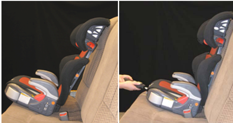
Figure 18. Placing the booster on the vehicle seat and applying force
