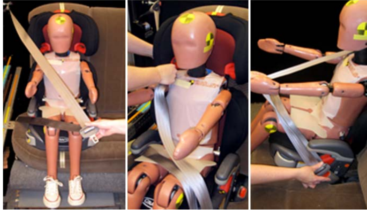
Figure 38. Initial deployment of the belt, routing the shoulder belt through the guide and buckling the belt
