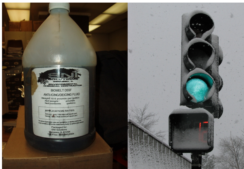
Figure 7. Chemical Deicer Fluid for Lens Application
