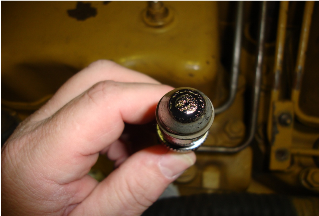
Nozzle Tip Condition Views - Cylinder #9 SSDG#2 Comparison
