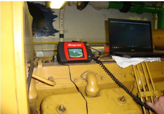
Borescope Instrument Setup and Inserted in Cylinder Nozzle Hole
