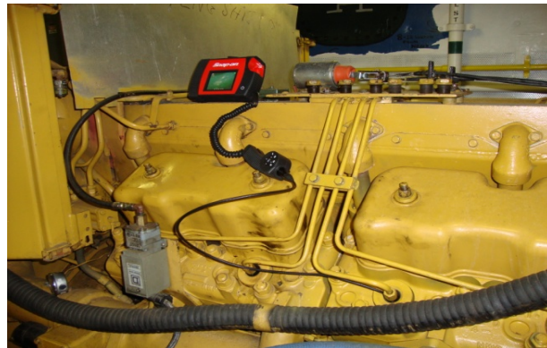
Borescope Instrument Setup and Inserted in Cylinder Nozzle Hole
