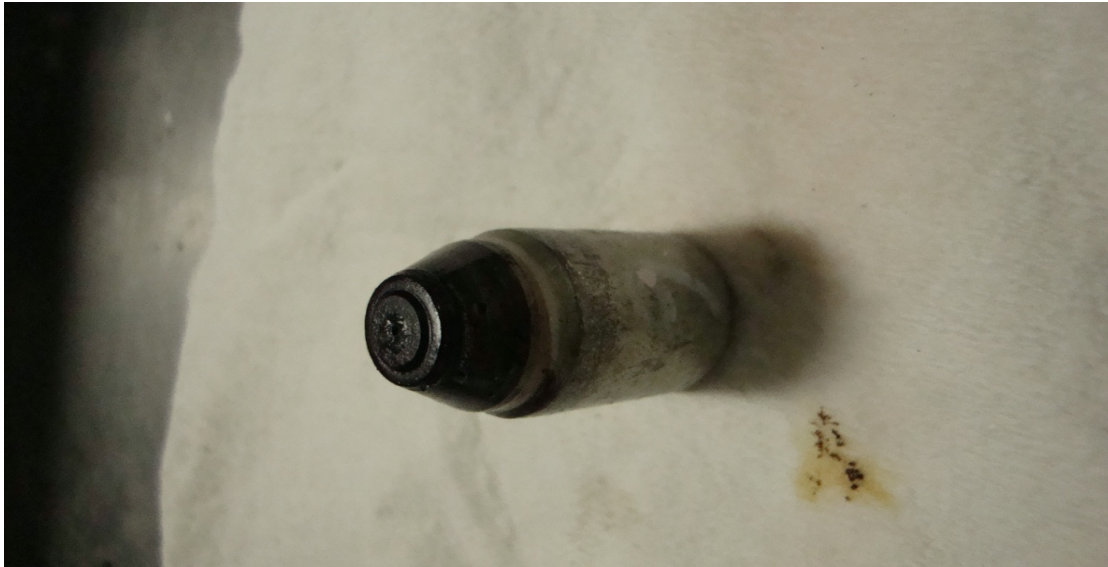
Nozzle Tip Condition Views - Cyl # 9 SSDG #4
