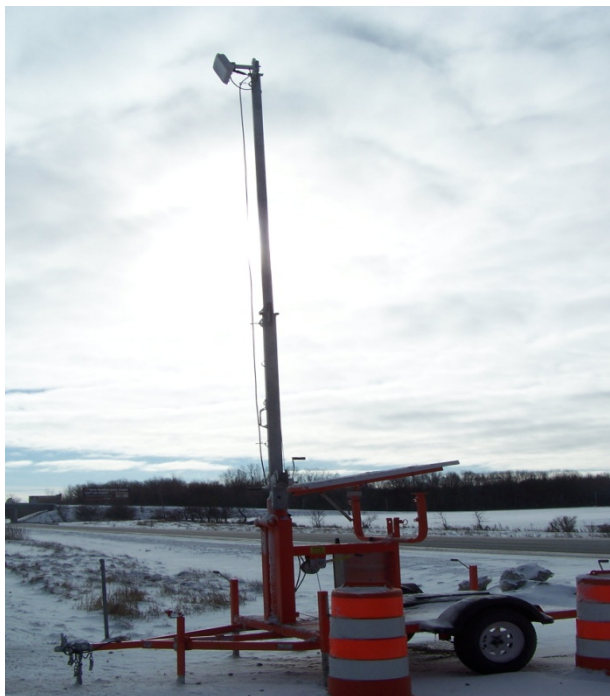
Figure MI-1. Speed sensor apparatus to determine regain time.
