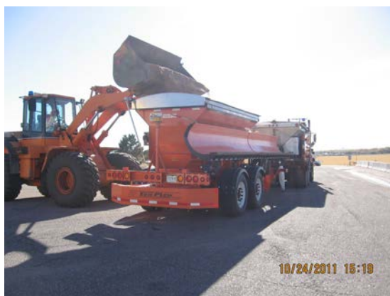
Figure CO-2. Tow plow being loaded with salt.
