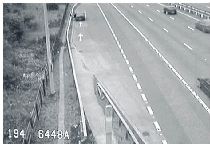
Figure 6. England: emergency refuge area in Birmingham (traffic travels on the left side on England's roadways).
