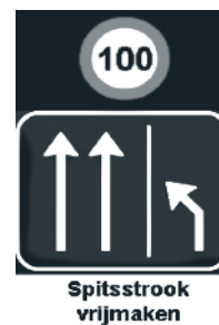
Hard shoulder running sign when lane is closing
