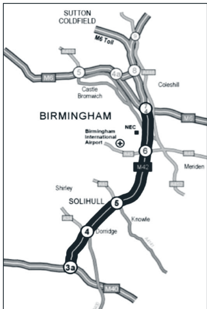
Figure 35. England: location of pilot test of hard shoulder running on the M42 in Birmingham. (19)
