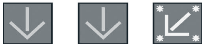
Overhead lane signal when lane is closing
