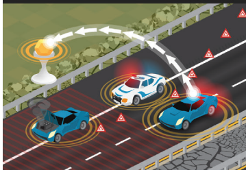
1. Vehicles slowing down due to crash (or at recurrent or non-recurrent congestion locations) broadcast speed, position, etc.
