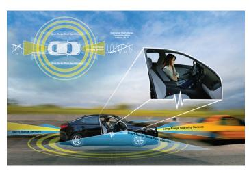
Automated vehicles use on-board sensors, cameras, global positioning, and telecommunications to help perform safety-critical driving functions such as steering, acceleration, and/or braking. To ensure full awareness of their surroundings, automated vehicles can leverage connected technology to communicate wirelessly with other vehicles and roadside infrastructure to improve safety, performance, and reliability.
