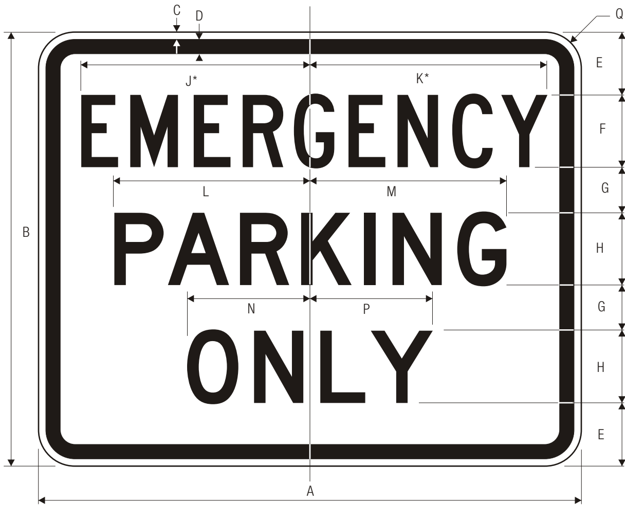
R8-4 EMERGENCY PARKING ONLY
