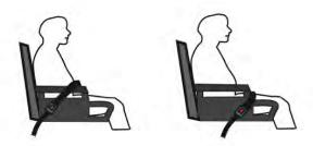
Improper positioning of a vehicle-anchored lap belt over (left) and in front of (right) wheelchair arm supports
