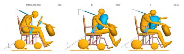
(c) - poor belt fit with steering-wheel air bag
