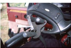
Tri-pin attached to lower steering-wheel rim
