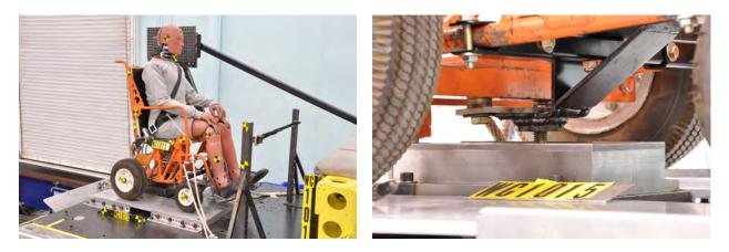
Figure 2.44 - Setup photos for a test of the surrogate docking-securement device (SDSD) with a 7.94-mm (5/16") thick hot-rolled steel plate used to secure the surrogate wheelchair (SWC) loaded with the midsize-male Hybrid III ATD restrained by a surrogate lap/shoulder belt and SWC-anchored lap belt
