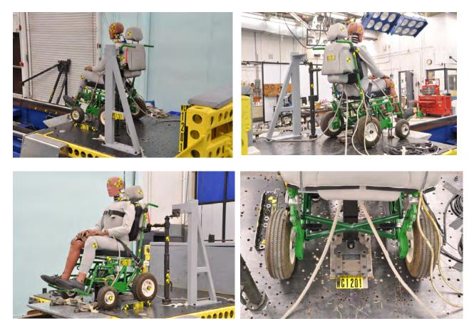
Figure 2.64 - Photos showing the setup of SWCF and midsize-male ATD for the first rear-impact sled test of the deployable Swedish head-and-back restraint system
