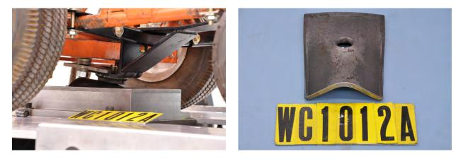
Figure 2.46 - Post-test photos showing plastic deformation of a 6.35-mm (1/4") thick hot-rolled steel plate still installed in the SDSD (left) and after removal from the SDSD (right)
