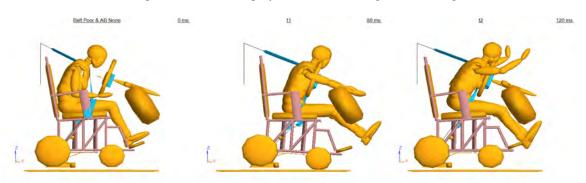
(d) - poor belt fit without deployment of the steering-wheel air bag
