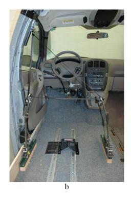
Figure 2.23 – Photos of a prototype of the pivoting-bar lap/shoulder belt restraint system installed in the static minivan buck
