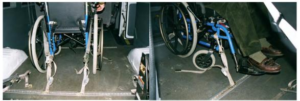
Damaged Wheelchair With Right Arm Support Bent Outward
