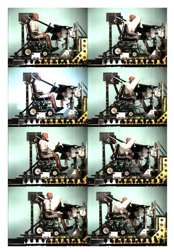
Figure 3.4 – Time-sequence frames from the side-view high-speed video from Test No. WC1022 with good belt fit and 12-ms air-bag deployment time, showing midsize-male ATD kinematics and interaction with the air bag
