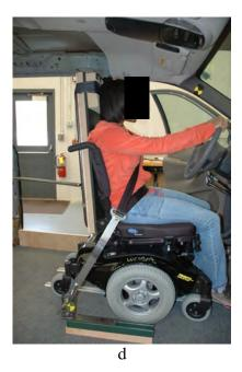
Figure 2.25 - Photos of BME students in power wheelchairs without arm supports evaluating the pivoting-bar lap/shoulder-belt restraint system used in the passive mode in the static minivan buck
