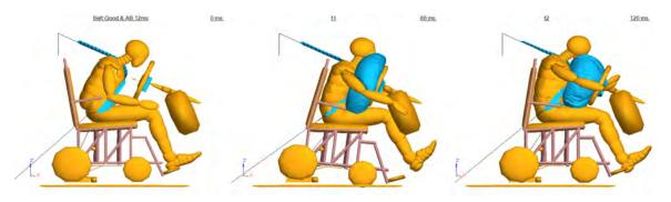
(a) - good belt fit with deployment of the steering-wheel air bag
