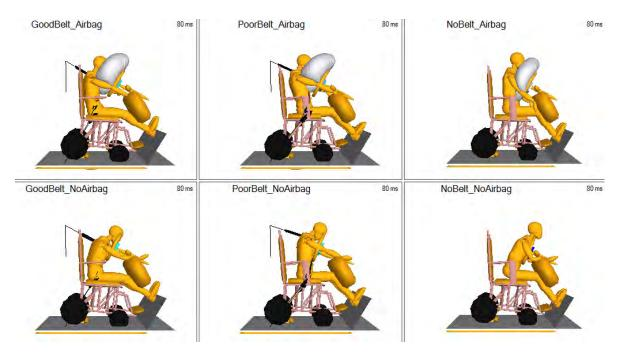
Figure 3.11 - Positions of the small-female ATD seated in the SWCF relative to the steering wheel, air bag, and knee bolster at 80 ms during a computer-simulated 48-kph, 20-g frontal impact – simulations are for good seat-belt fit (left), poor (loose) seat-belt fit (middle), and no seat belt (right) and for air-bag deployment at 12 ms (upper) and no air bag
