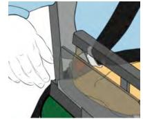
Lap belt threaded into opening between the seat and back support to achieve proper positioning low on the pelvis
