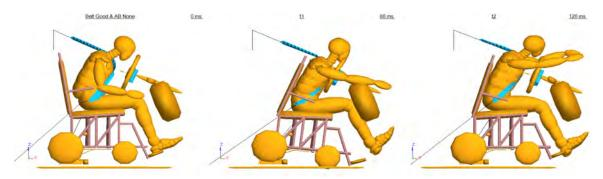
(b) - good belt fit without deployment of the steering-wheel air bag
