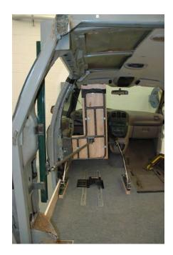
Figure 2.57 - Photos of a BME student-designed deployable vehicle-mounted head-and-back restraint system installed in the static minivan buck – the photos on the left show the head-and-back restraint in the stored position while the photo on the right shows the head-and-back restraint in the deployed position
