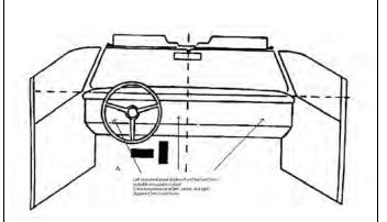
Left instrument panel displaced and fractured from probable occupant contact with lower extremities.
