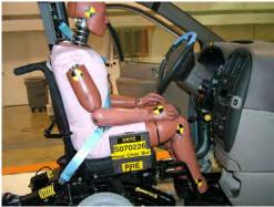
Figure 2.18 - Photos of pretest setups for two TRC sled tests – the photo on the left shows the inboard buckle of the OEM seat belt anchored to the vehicle floor by means of a cable stalk, and photo on the right shows an aftermarket lap/shoulder belt with the lap belt anchored to the back of the wheelchair near the docking-securement adaptor
