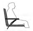
Proper positioning of a vehicle-anchored lap belt with wheelchair arm supports that are attached to the back-support posts and completely open at the front and underneath
