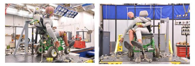
Figure 2.72 - Post-test photos from the fourth rear-impact test of the modified Swedish deployable vehicle-anchored head-and-back restraint system
