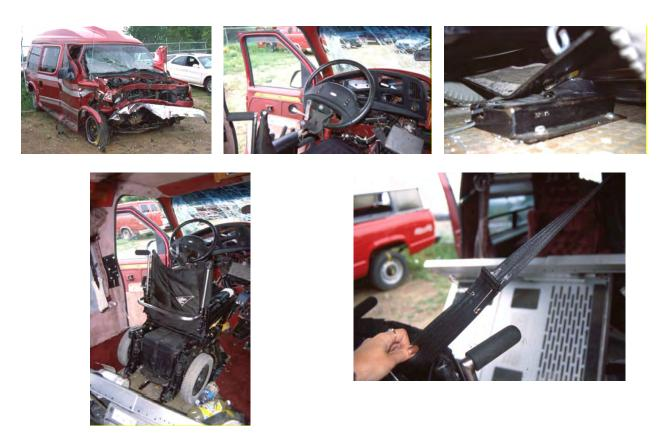
Figure 1.2 - Exterior and interior photos of a full-size van operated by a driver seated in a power wheelchair who sustained fatal chest and abdomen injuries in a severe frontal crash
