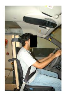
Figure 2.58 – Early prototype of the BME student-designed deployable vehicle-mounted head-and-back restraint in the deployed position behind a student seated in a wheelchair
