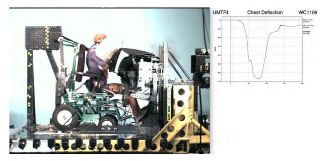
Figure 3.7 - Side-view photo at PEAK CHEST DEFLECTION from high-speed video for Test No. WC1109 with the small-female ATD restrained by loosely fitting lap/shoulder belt and an air-bag deployment time of 42 ms
