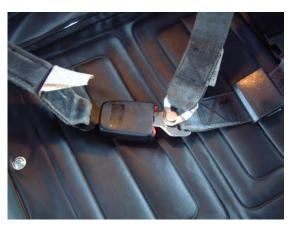
Lap-belt buckle with lower end of shoulder belt attached
