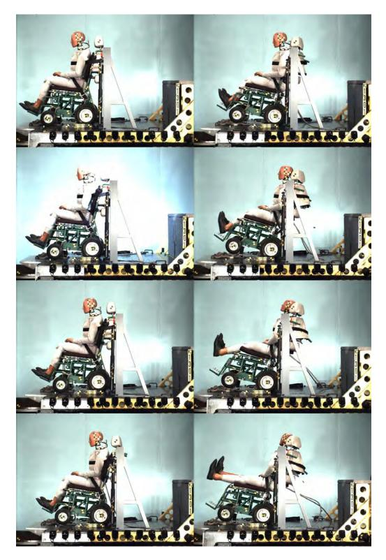
Figure 2.75 – Time-sequence frames from the side-view high-speed digital video of the fourth rear-impact sled test of the Swedish deployable vehicle-anchored head-and-back restraint system – note that there is no rearward rotation of the SWCF
