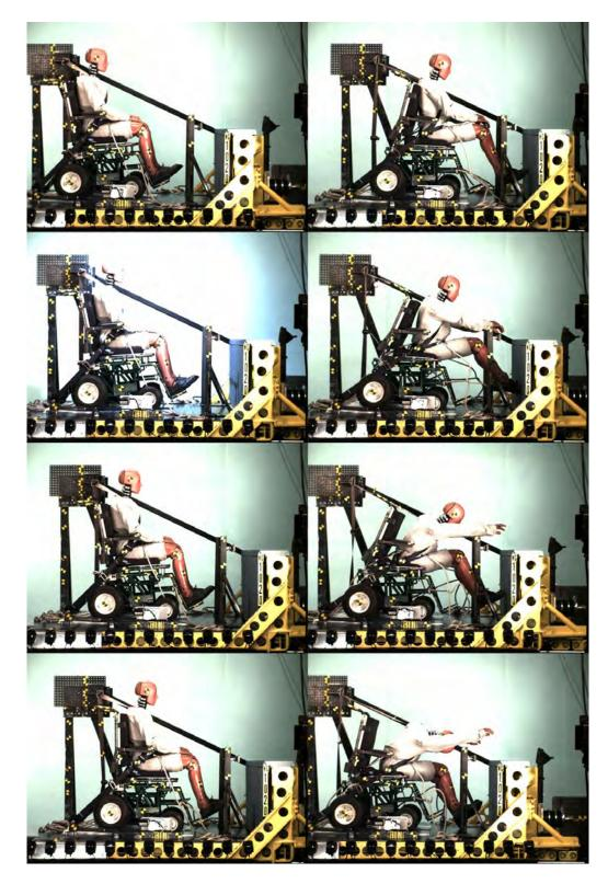
Figure 2.53 – Time-sequence frames from the side-view high-speed video of a 48-kph, 20-g frontal-impact sled test of the SBDS with an OEM lap/shoulder belt and upper-shoulder belt D-ring and ELR retractor
