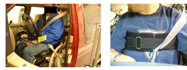
Figure 2.13 - Photos showing typical positioning of the shoulder belt nearly off (left) or completely off (right) the driver's outboard shoulder
