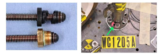
Figure 2.70 - Broken plastic drive nut (upper part of photo on left) on screw-motor actuator and slippage in curved slots at the base of the Swedish head-and-back restraint post (right) that were significant contributors to the poor performance of the Swedish deployable vehicle-anchored head-and-back restraint system in the second sled test
