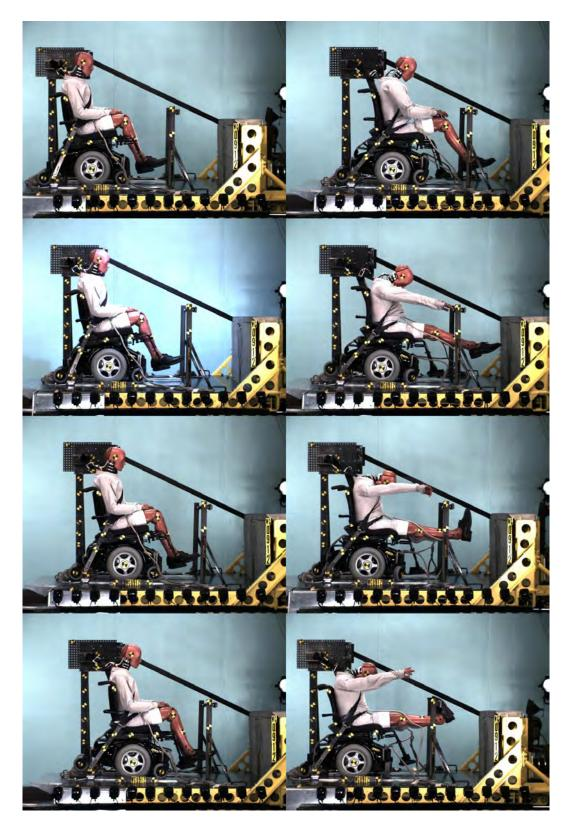
Figure 2.27 – Time-sequence frames from the side-view high-speed digital video for the third 48-kph, 20-g sled test of the pivoting-bar lap/shoulder belt restraint system
