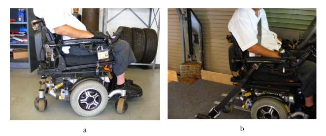
Figure 2.55 - Power wheelchair retrofitted with open-front cantilevered arm supports (a) and driver using a passive lap/shoulder belt with the seat-belt deployment system showing good fit of the lap belt low and in contact with the pelvis (b)
