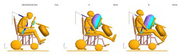
(a) - good belt fit with deployment of the steering-wheel air bag
