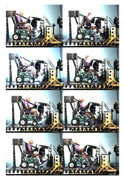
Figure 3.5 - Time-sequence frames from the side-view high-speed video of Test No. WC1109 with poor (loose) belt fit and 42-ms airbag deployment time, showing small-female ATD kinematics and interaction air bag
