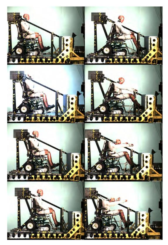
Figure 2.52 - Time-sequence frames from the side-view high-speed video of a 48-kph, 20-g frontal-impact sled test of the SBDS with a surrogate three-point lap/shoulder belt and fixed upper shoulder-belt anchor point
