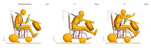
(b) - good belt fit with no steering-wheel air bag
