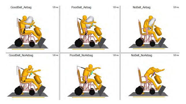
Figure 3.12 - Positions of the small-female ATD seated in the SWCF relative to the steering wheel, air bag, and knee bolster at 120 ms during a computer-simulated 48-kph, 20-g frontal impact – simulations are for good seat-belt fit (left), poor (loose) seat-belt fit (middle), and no seat belt (right) and for air-bag deployment at 12 ms (upper) and no air bag
