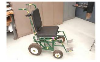
Figure 2.17 - Surrogate wheelchair frame (SWCF) used in tests to evaluate front- and rear-impact restraint systems to evaluate restraint systems in both front and rear impacts
