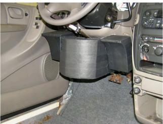
Figure 2.30 - Photo of a prototype close-proximity knee restraint installed in the static minivan buck
