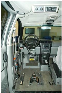
OEM seat belt being used in the active mode
