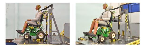
Figure 2.77 - Pre-test photos of the manufacturer' revised design of the Swedish deployable vehicle-anchored headand-back restraint system
