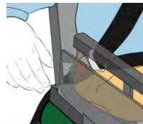
Lap belt threaded into opening between the wheelchair seat and back support to achieve proper positioning low on the pelvis
