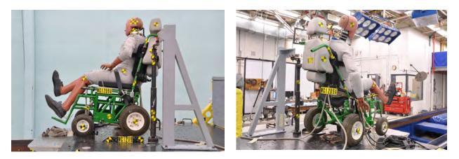
Figure 2.71 - Post-test photos from the third rear-impact test of the modified Swedish deployable vehicle-anchored head-and-back restraint system
