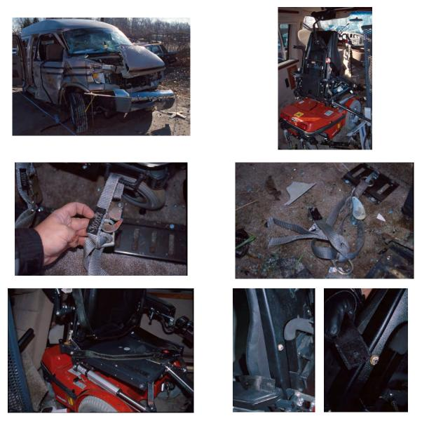
Figure 1.4 - Exterior and interior photos of a van driven by a male driver seated in a power wheelchair that was involved in a frontal crash into the side of the cab and box of a dump truck at a four-leg intersection
