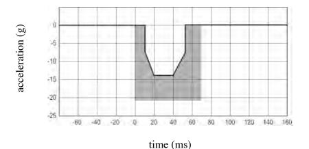
Figure 2.59 - Deceleration corridor (shaded area) for proposed rear-impact testing of wheelchairs in WTS standards now under development
