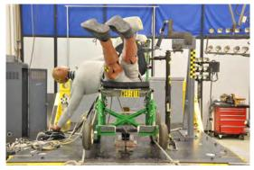
Figure 2.78 - Post-test photos of the Swedish manufacturer's modified design of the deployable vehicle-anchored head-and-back restraint system
