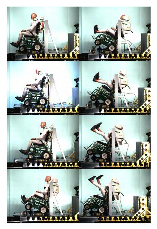
Figure 2.68 – Time-sequence frames from the side-view high-speed digital video of the second rear-impact sled test of the Swedish deployable vehicle-anchored head-and-back restraint system – note the rearward rotation of the SWCF
