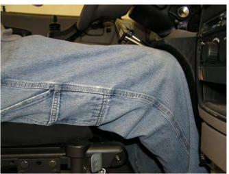
Figure 2.31 - Position of the right knee relative to a prototype contoured close-proximity knee restraint in the static minivan buck
