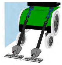
Illustration of securement loops attached to the back of a wheelchair frame to provide easily accessible places for attaching tiedown hooks
