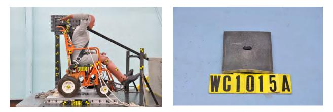
Figure 2.45 - Post-test photos for the sled test of Figure 2.44 showing the degree of plastic deformation of the 7.94mm (5/16") thick hot-rolled steel plate on the right
