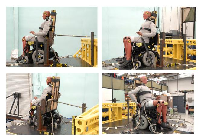
Figure 2.61 - Post-test photos of the second rear-impact sled test of a BME student-designed vehicle-mounted head-and-back restraint
