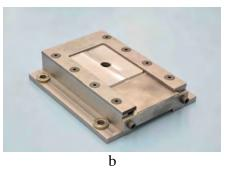
Figure 2.43 - Photos of the final design of the surrogate docking-securement device: a) disassembled with two thicknesses of deformable/replaceable plates; b) assembled
