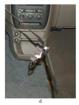
Figure 2.24 – Additional photos of a prototype of the pivoting-bar lap/shoulder belt restraint system installed in the static minivan buck
