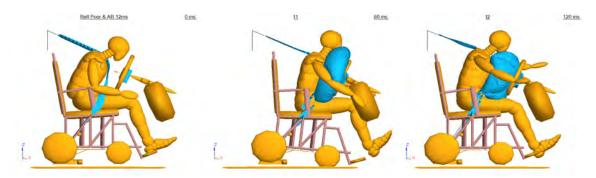
(c) - poor belt fit with deployment of the steering-wheel air bag
