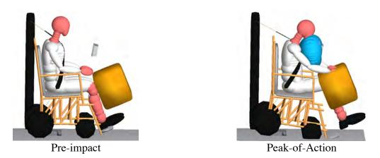
Figure 2.35 - MADYMO simulation for an unbelted midsize-male ATD restrained by a two-point shoulder belt, a steering-wheel air bag, and a 100-mm deep, 50 N/mm close-proximity knee restraint added to the production knee restraint
