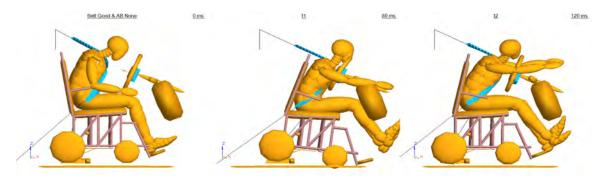
(b) - good belt fit with no steering-wheel air bag
