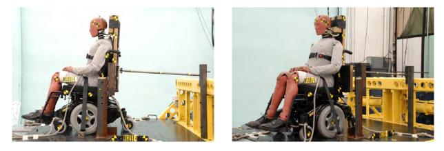
Figure 2.60 - Pre-test photos for the second rear-impact sled test of a BME student-designed vehicle-mounted head-and-back restraint
