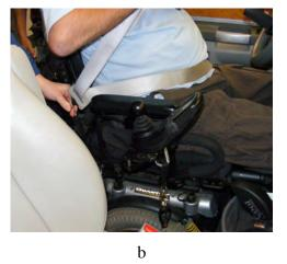
Figure 2.54 – Closed-front arm supports on power wheelchair (a) and poor positioning of passive lap belt over closed-front arm supports and on the abdomen (b) with the driver ready for travel in his personal vehicle
