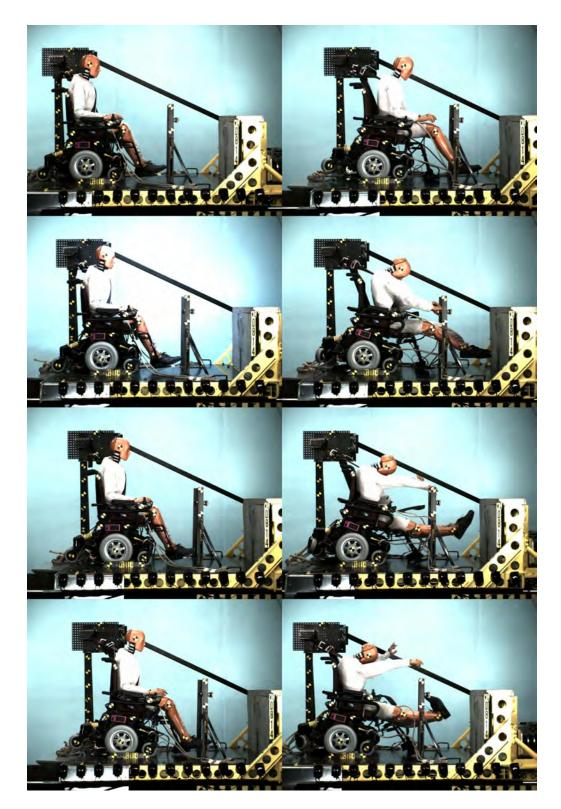
Figure 2.21 - Side-view time-sequence photos from the side-view high-speed digital video of the second test of a BME-student prototype lap/shoulder belt restraint system with wheelchair-anchored lap belt
