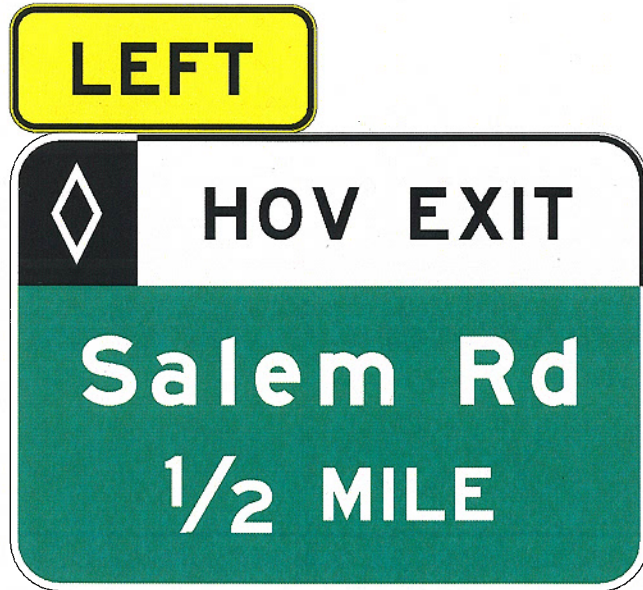
Fig. 1. Example of an Advance Exit Guide sign for a direct exit from a preferential lane.
