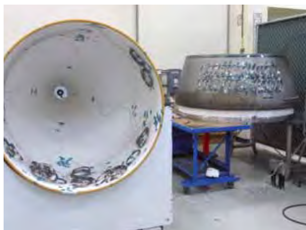
Under FAA's Continuous Lower Energy, Emissions and Noise (CLEEN) Program, Boeing developed the Ceramic Matrix Composite (CMC) acoustic engine nozzle to reduce fuel burn, emissions and noise. CMC material (shown as white color) allows operation at higher temperatures, leading to more efficient engines. The CMC nozzle and center body above are instrumented for ground tests on a Trent 1000 engine, scheduled for December 2012. (Image courtesy of Boeing.)
