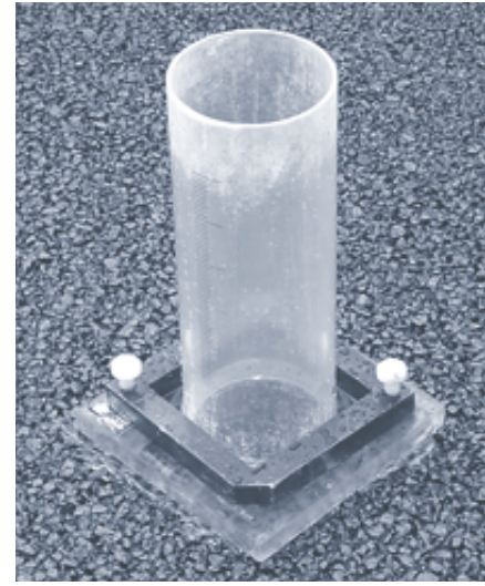
Figure 12. Permeability testing of recycled mix.
