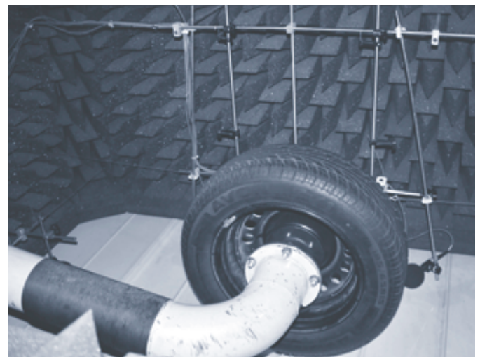
Figure 6. Danish noise-measurement trailer.
