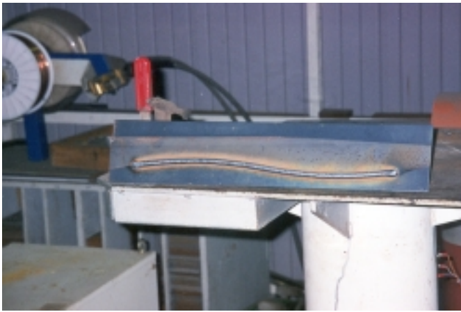
Figure 7. Robot demonstrating high-speed rotating arc welding at NKK Corp.'s Tsu Works plant in Japan.
