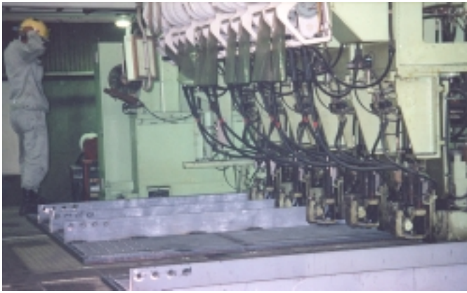
Figure 1. Flange panel fabrication line at Sakai plant of Matsuo Bridge Co., Ltd., in Japan.
