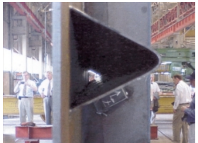
Figure 45. Closed web stiffener used in Italy.
