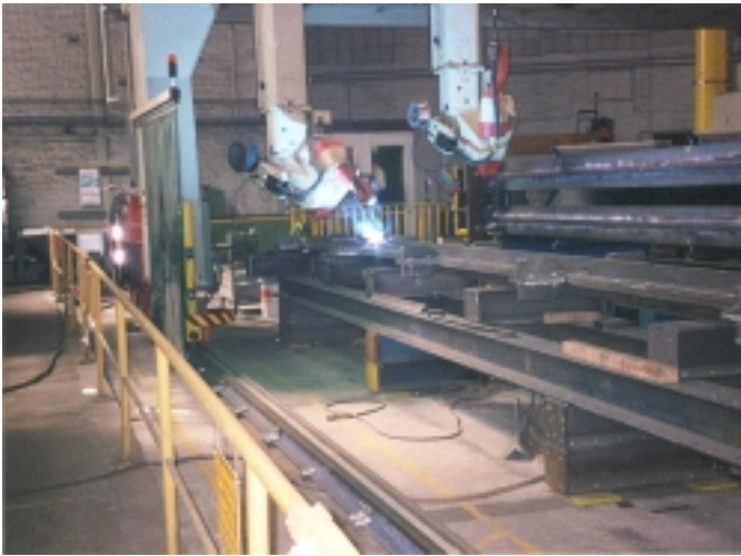
Figure 19. NC robotic welding at Krupp Stahlbau Berlin plant.
