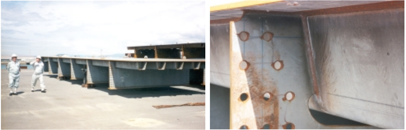
Figure 15. Fabricated orthotropic deck sections at Shikoku plant.
