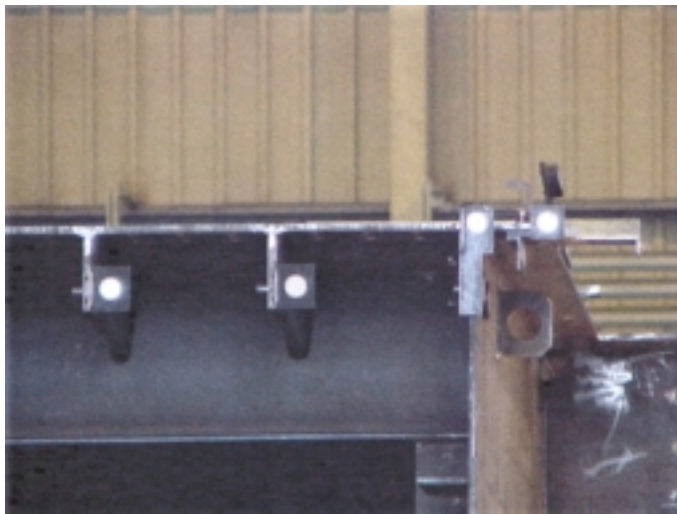
Figure 26. Targets for CATS geometry checking system at Yokogawa Bridge Corp. in Japan.
