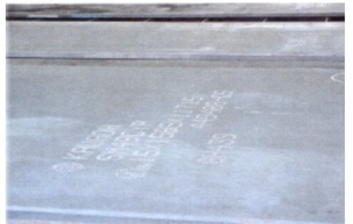
Figure 30. Mill-coated steel plate used in Japan.
