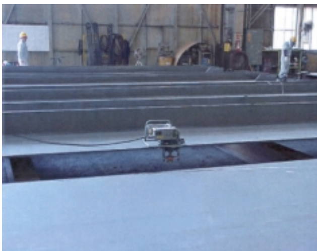
Figure 41. Edge grinding equipment in Japan.
