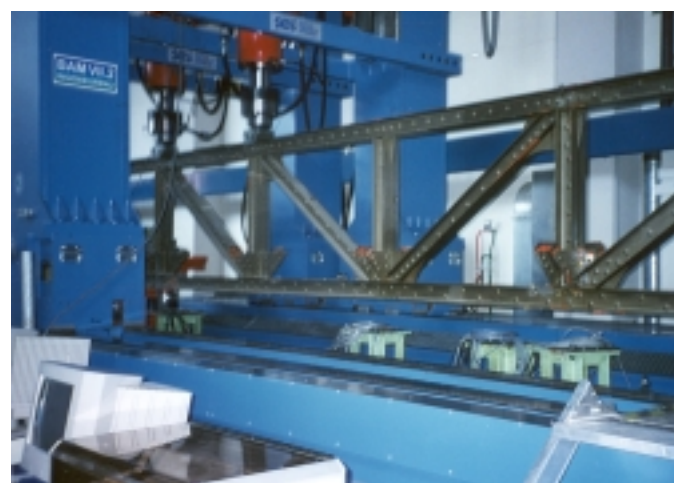
Figure 18. Tests on old, riveted truss-girder bridge members under cyclic loading by BAM in Germany.
