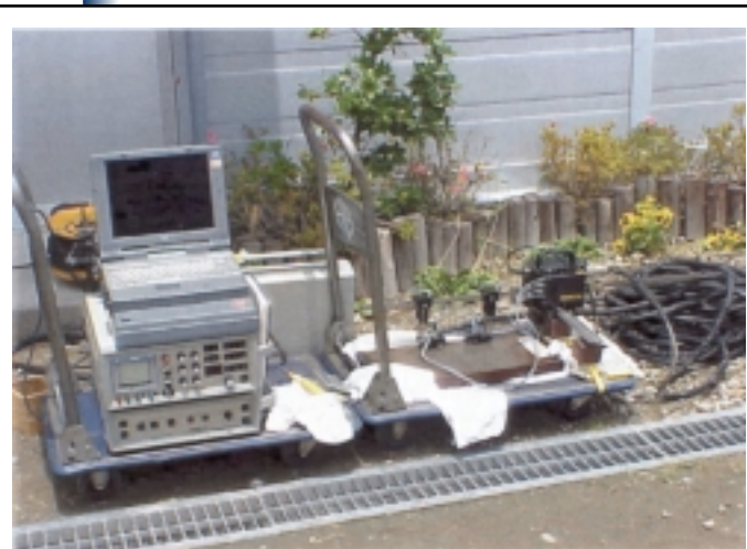
Figure 27. Automated ultrasonic inspection equipment used in Japan.
