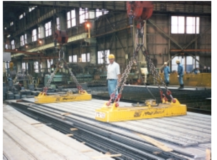
Figure 4. Cranes with lifting magnets move multiple flange plates at Yokogawa plant.
