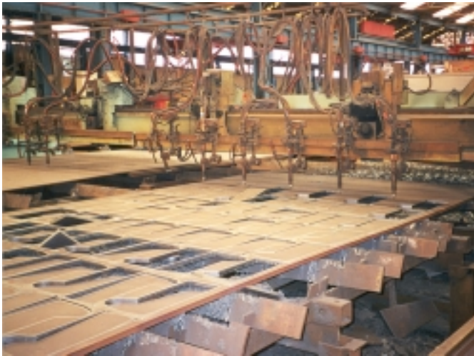
Figure 23. NC gas and plasma cutting machines at Fairfield-Mabey's fabrication plant in Chepstow, Wales.
