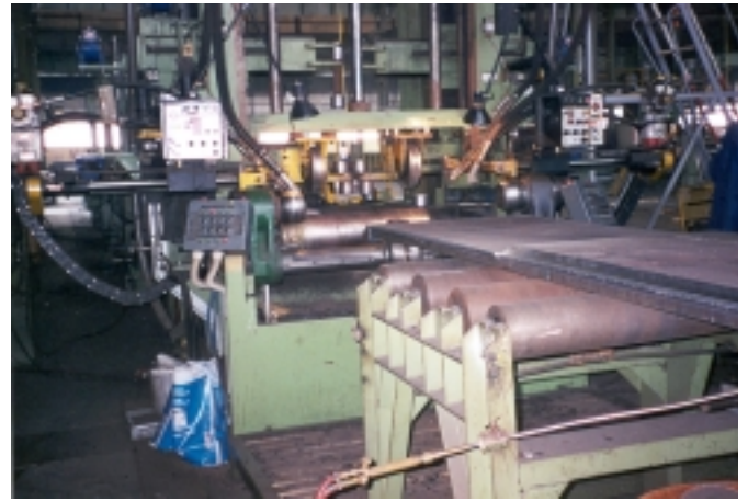
Figure 16. Automated handling and assembly of welded beam members by machines designed and built by Cimolai in Italy.
