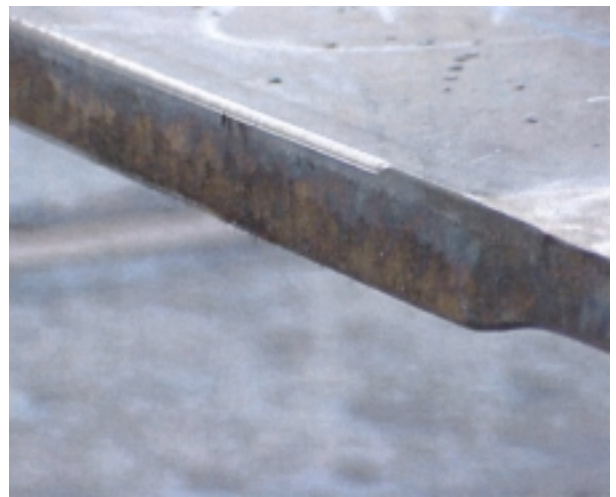
Figure 42. Ground edge, as used in Japan.
