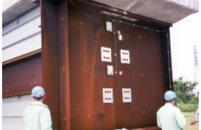
Figure 8. Seaside exposure test by Tsu Works of a partial, full-scale seaside weathering steel bridge with small-scale plate samples.
