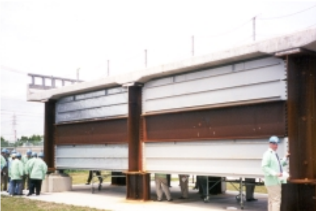
Figure 8. Seaside exposure test by Tsu Works of a partial, full-scale seaside weathering steel bridge with small-scale plate samples.
