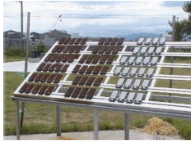
Figure 29. Weathering steel and primer corrosion test samples in Japan.
