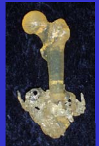
Virtual model processed and "printed" into a three-dimensionally accurate physical model
