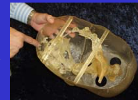
Virtual model processed and "printed" into a three-dimensionally accurate physical model
