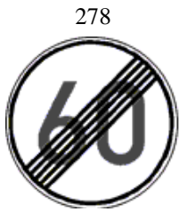
End of Speed Limit. Indicates the end of a speed-limit zone (sign 274).
