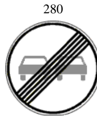
End of No-Passing Zone. Indicates the end of a no-passing zone for motor vehicles (sign 276).
