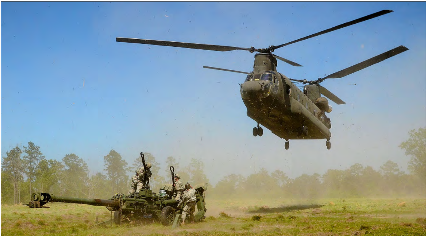
A CH-47 Chinook from the Mississippi National Guard flies on final approach to conduct a sling load operation with Section 2, A Battery, gun crew of the Alabama Army National Guard 1-117th Field Artillery. The members of Section 2 are responsible to connect two ropes, connecting four points, to the CH-47. (Photo by Staff Sgt. Christopher Davis)
