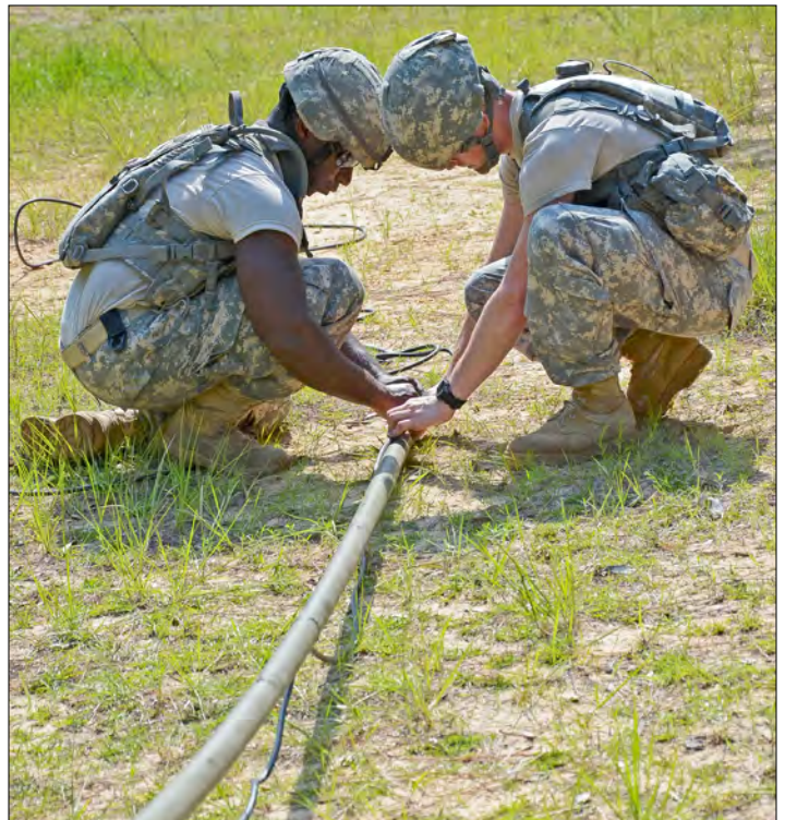
Sgt. Markus Saunders and Pvt. 1st Class. Seth Bayer, both from the 152nd MP Co, set up an Antenna Group OE- 254/GRC system to help run a communications relay for MP teams throughout the Alabama Army National Guard training grounds on Eglin Air Force Base, Florida. (Photo by Staff Sgt. Christopher Davis)
