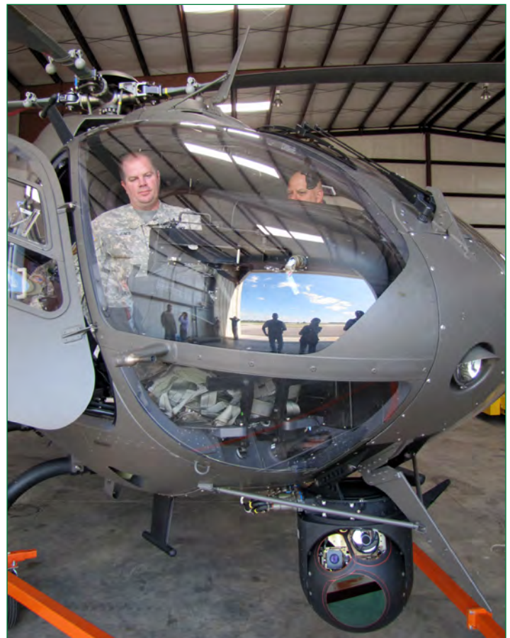
National Guard pilots from four states are now training on the UH-72A Lakota Security & Support variant at the Madison County Executive Airport in Alabama. The aircraft provides long-range electro-optical sensors and the ability to record and downlink data. (Courtesy photo)
