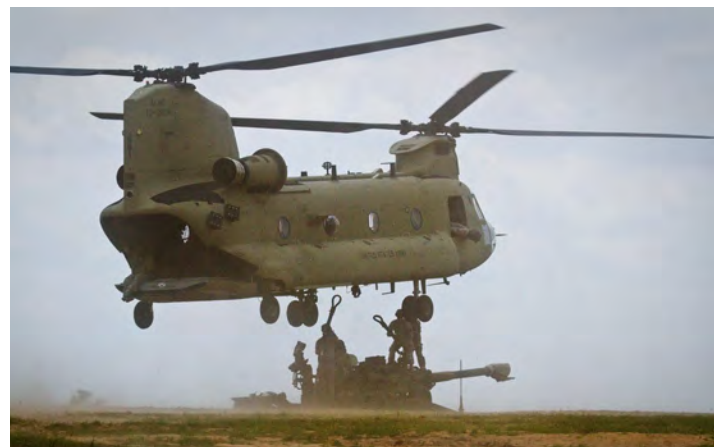
Soldiers attach a Howitzer long-gun to a Chinook helicopter for transportation. (Contributed photo.)
