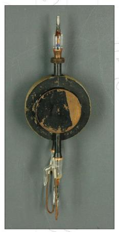
When the members of the Tizard Mission arrived in Washington DC in September 1940, they carried with them a black metal deed box that contained, among other things, a special vacuum tube known as a cavity magnetron—E1189 Serial No. 12. Manufactured by the General Electric Company Ltd. at Wembley in North London, the magnetron was the result of several years of research and development aimed at creating a viable and powerful source of microwaves for radar systems.
