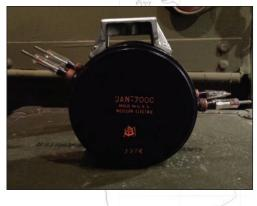
magnetrons were the Western Electric WE 700 series. Thirty magnetron prototypes were manufactured by Western Electric based on the E1189. This is number 6, which was given to the engineering manager of the Westinghouse radio division in Baltimore, Maryland. The unit subsequently was passed to the head of the radar section and then to one of the founding board members of the National Electronics Museum.
