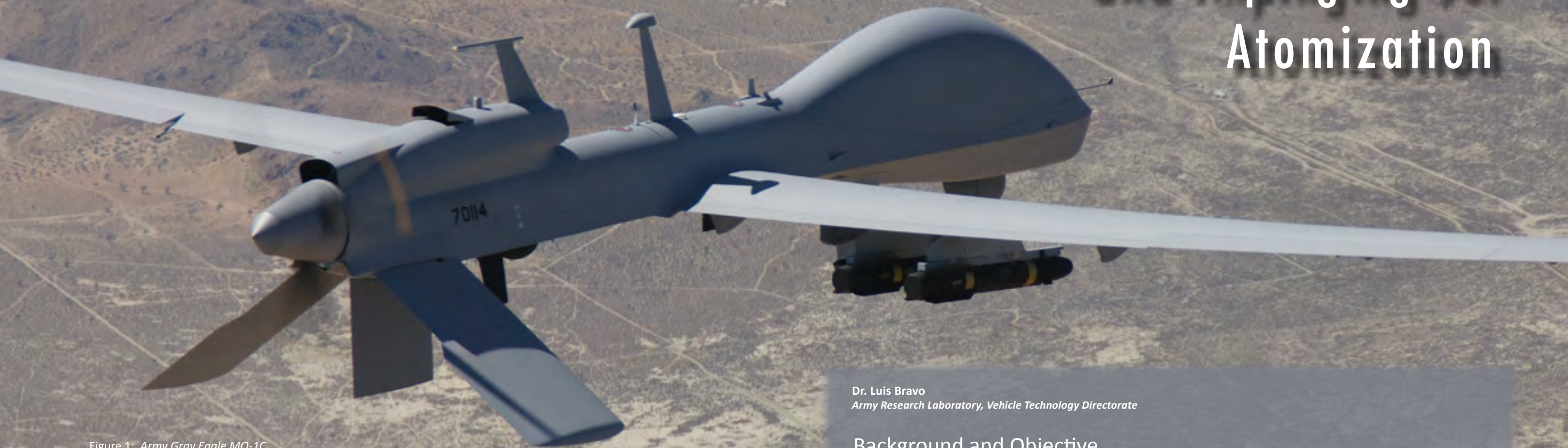
Figure 1: Army Gray Eagle MQ-1C, powered by turbo-charged diesel engine (160hp) on mission. (Photo courtesy of the US Army Acquisition Support Center)
