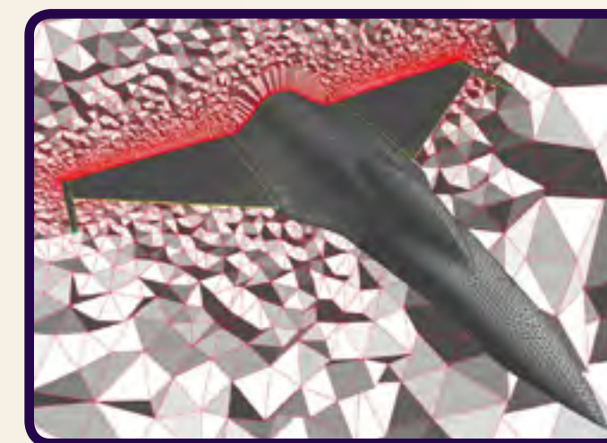
CREATE-MG Boundary-layer meshes for flow around model aircraft
