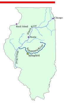
In the last 20 years, the sediment has started to deposit in the main channel of the Illinois River, impacting navigation and increasing dredging costs downstream of the confluence with the Sangamon River. The source(s) of sediment (overland or in channel) in the Sangamon River is unknown.
