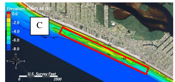
A) Location of nearshore placement in the form of a “Swash-zone Berm” in Perdido Key, Pensacola, FL; B) Location of nearshore placement in the form of a shallow mound in Egmont Key, Tampa, FL; C) Bathymetric map of the Ft. Myers Nearshore Berm Placement in 2009.
