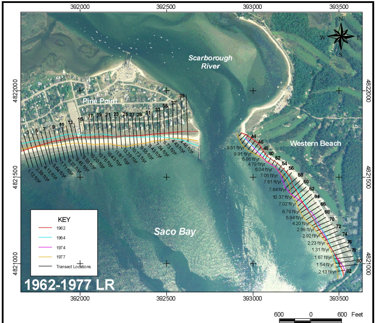
Figure C-2.2 Map of transect locations and shoreline movement rates from 1962-1977 for Pine Point and Western Beach, ME. Linear regression rates display a pattern of mild to moderate rates of shoreline accretion.
