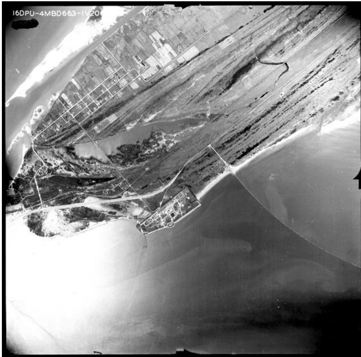
Figure 9. Bolivar Peninsula, near the mouth of Galveston Bay, Texas, January 1952. The line extending to the lower right is the Galveston north jetty. A fillet has not built up against the jetty, but shoals have accumulated further to the northeast.
