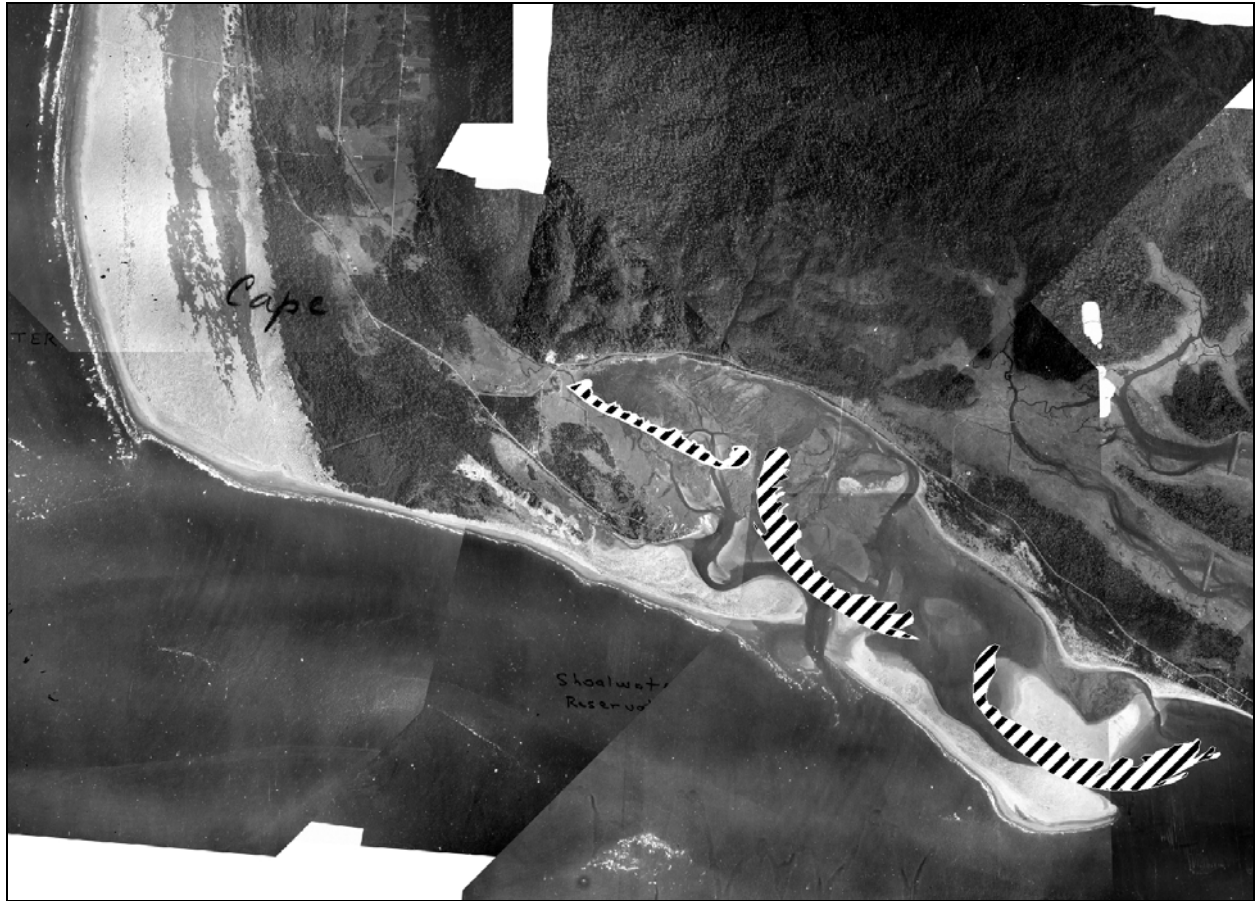
Figure 10. North Willapa Bay, Washington State. This mosaic consists of six frames flown on September 19, 1945. These have been photogrammetrically rectified to create a map projection. The three islands (hatched polygons) were traced from an October 12, 2000, orthophoto. The shoreline retreat at the spit in the center of the map was 1,100 m, or 20 m/year. (Original photographs, BEB archives, mosaic courtesy of Washington State Department of Ecology).
