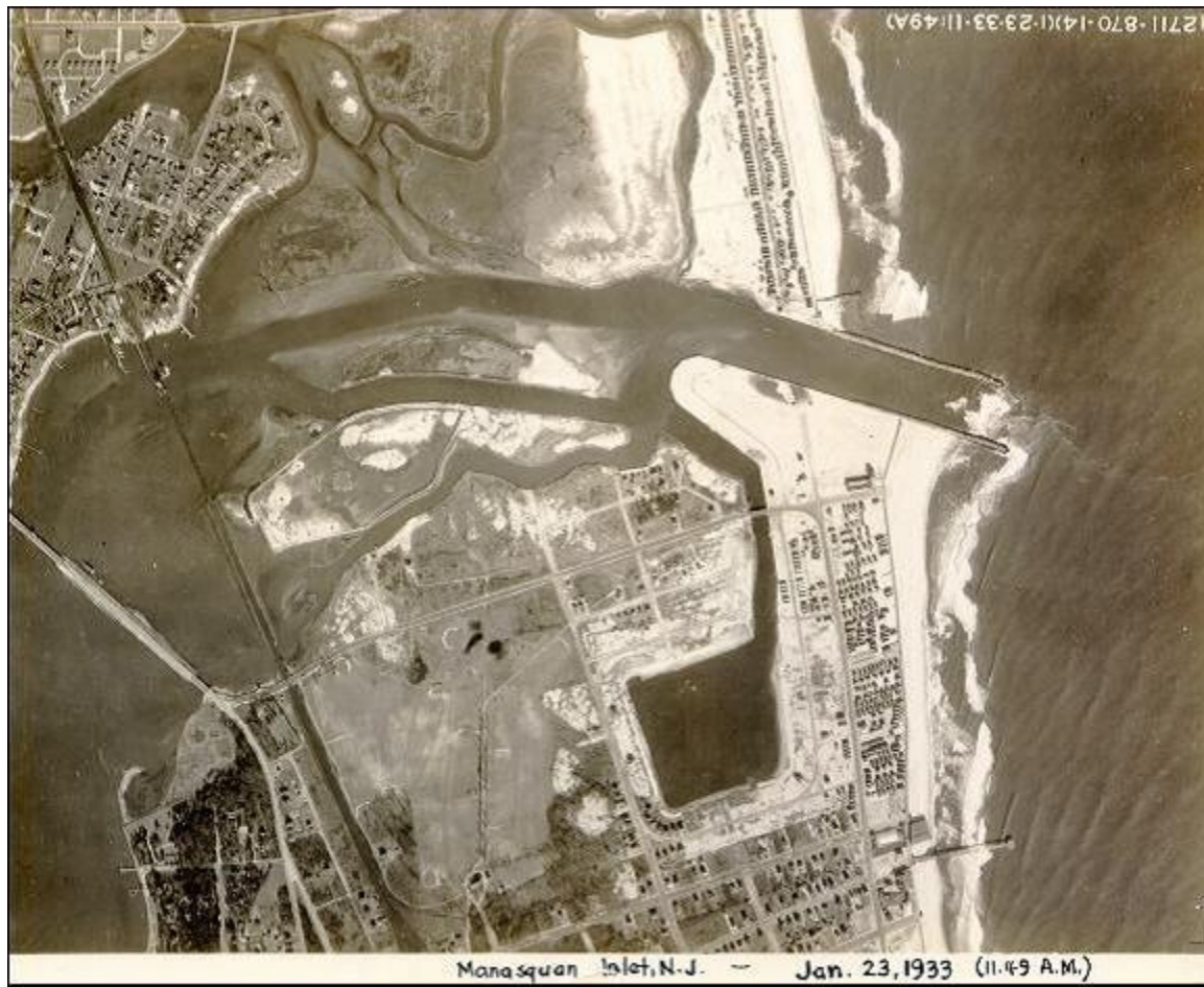
Figure 8. The recently opened Manasquan inlet, January 23, 1933. The south fillet has almost filled with sand, and developers have built a road seaward of the seaward-most row of cottages in Figure 7.
