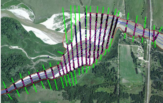
Figure 8. Surveyed cross sections and HEC-RAS model cross sections superimposed on an aerial photograph of Spencer Reservoir.
