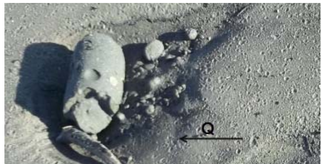
Figure 7. Clay roller, a chunk of a clay lens, undermined and sloughed into the flow field, transported into a cylindrical rolling clast (about 10 cm long).
