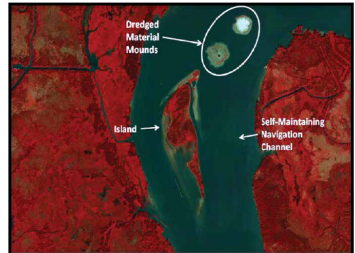
Figure 1: December 2011 aerial infrared photograph of the Atchafalaya River island after multiple years of upstream mounding of dredged material. The island's formation has reduced the overall cross sectional area of the river, increasing river flow through the navigation channel to the east sufficient to reduce shoaling and maintenance dredging requirements.
