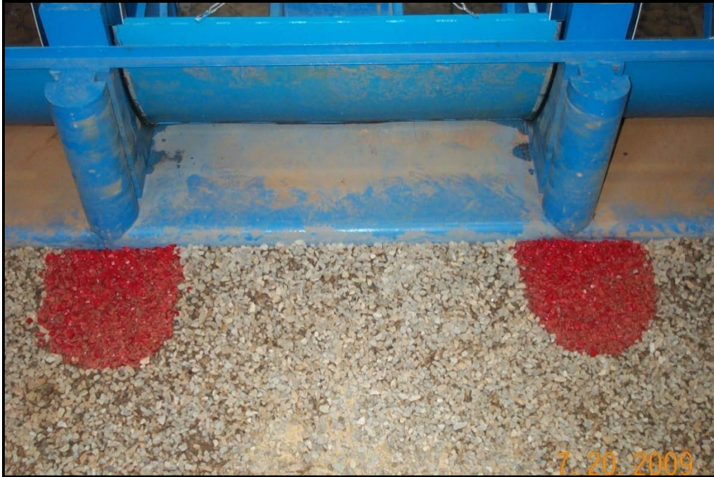
Figure 8 - Upstream pre-test conditions for a 23 ft. center gate opening Upper pool = 419 ft., original stone placement test
