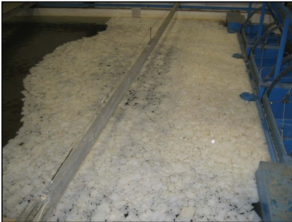
Figure 17 - Mechanically packed acrylic ice upstream of the gates
