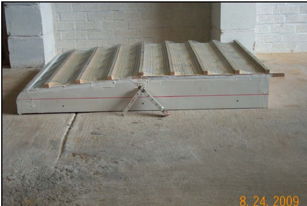
Figure 6 - Wooden raft used to simulate upstream ice
