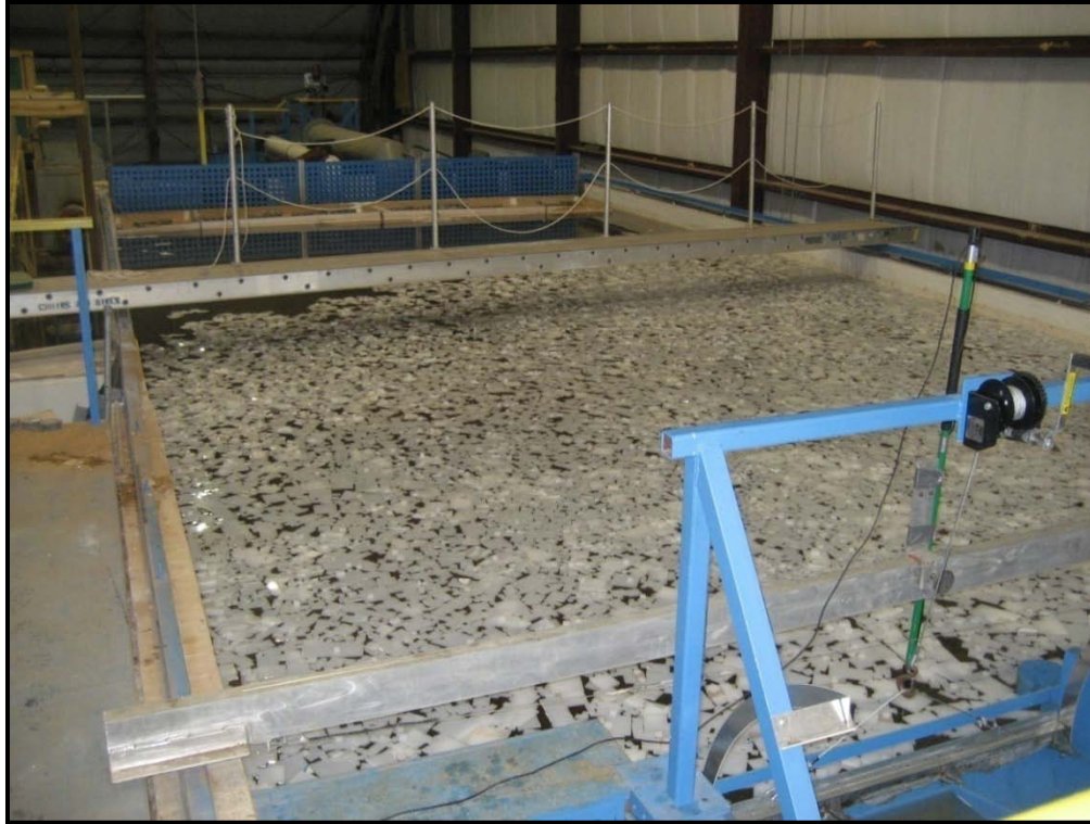
Figure 16 - Acrylic ice pieces in the flume upstream of the gates
