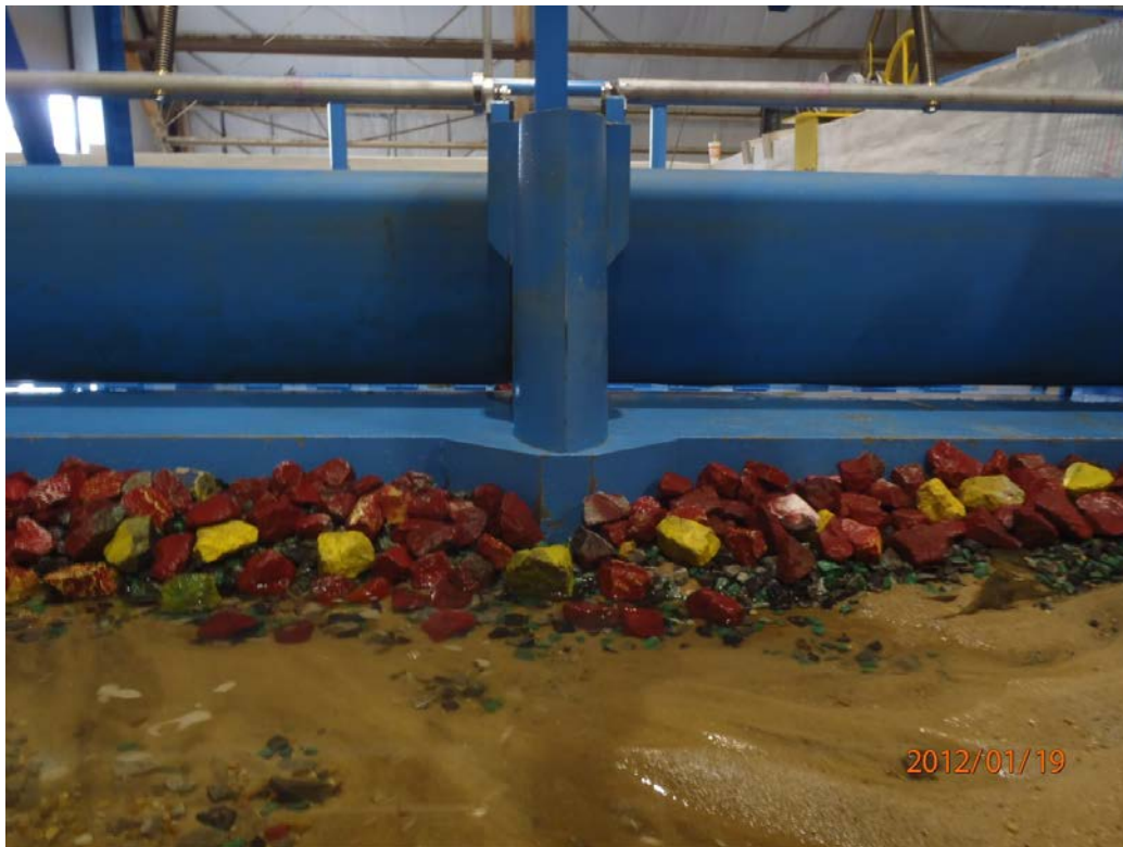
Figure 10 - 7 ft center gates, 20 ft ice raft draft
