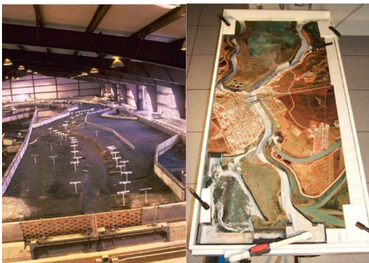
(a) Large coal bed model, Dogtooth Bend, scale 1:400 horizontal, 1:100 vertical, and (b) HSR model, Atchafalaya River, scale 1:7200 Horizontal, 1:1200 Vertical.
