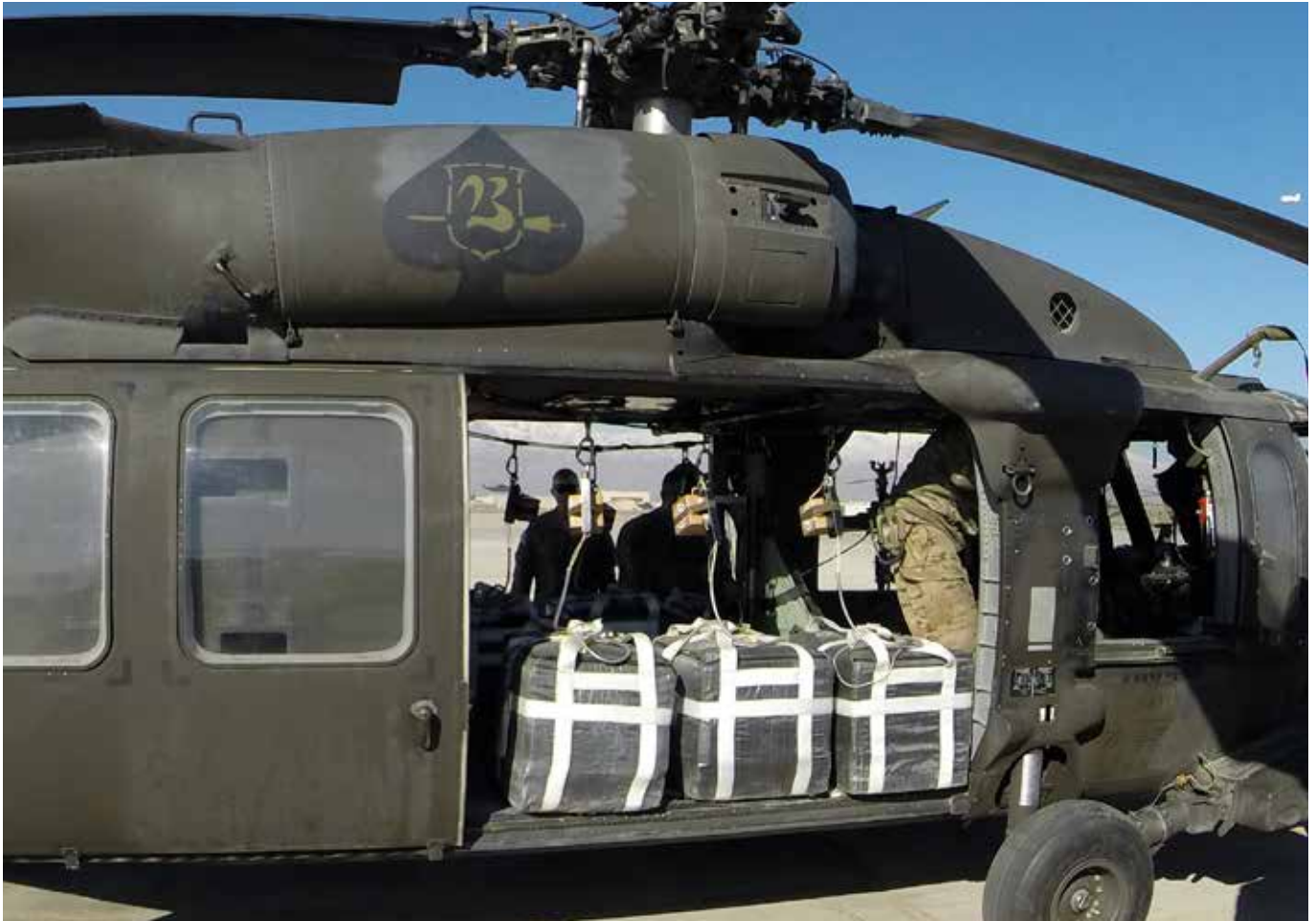
Three enhanced speed bag systems are rigged on a UH-60 Black Hawk helicopter and ready for resupply Jan. 31, 2013, at Bagram Airfield, Afghanistan. (Photo by Sgt. 1st Class Samuel M. Bright)
