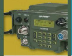
A wireless voice and data radio that allows troops to exchange large amounts of tactical data, such as video and biometrics. The radio can support small-unit operations and connect the tactical edge with forces at company level and above.
