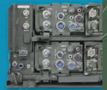
The primary radio the Army uses for voice communications in the field today. With configurations including manpack, vehicular (both low and high power), and airborne models, more than 500,000 SINCGARS have been fielded.
