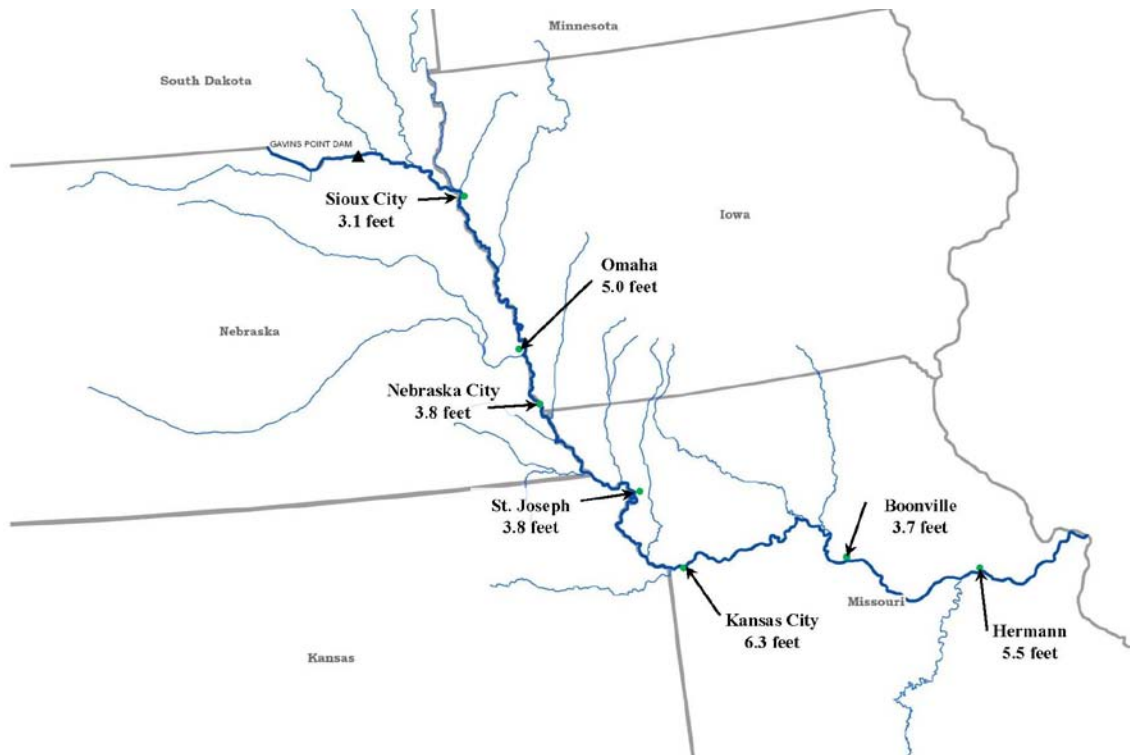
Figure 9B. Missouri River Peak Stage Reductions Due to Corps Reservoir Operations in 2010
