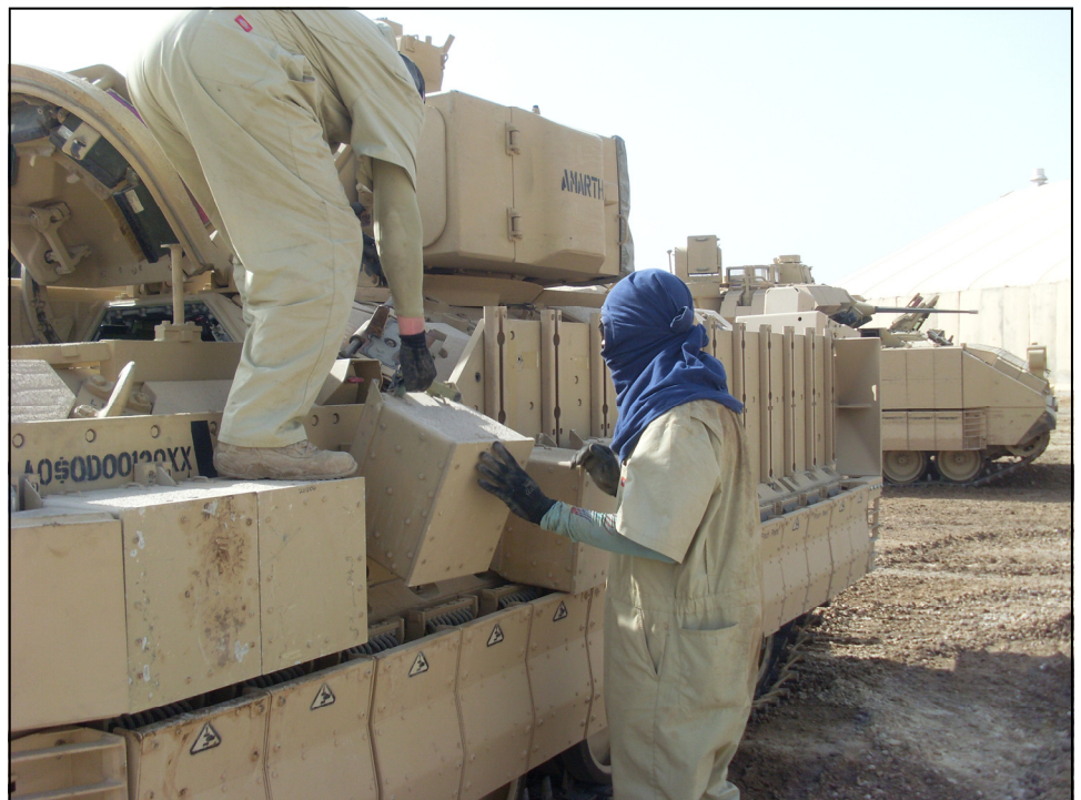
BAE Systems field support representatives install Bradley Reactive Armor Tile II kits at Contingency Operating Station Kalsu.
