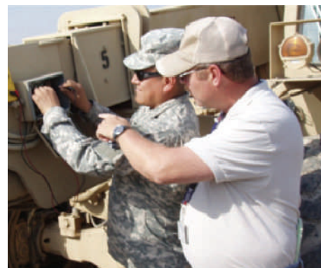
LAR Jordan is showing SSG Pino, B Company, 3rd BSB Maintenance Supervisor, how to check the boom wiring harness for shorts on a 10K ATLAS forklift.
